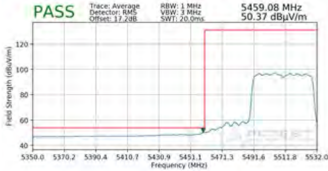
Plot 7-414. Radiated Lower Band Edge Plot MIMO (Average – UNII Band 2C – 484 Tones)
