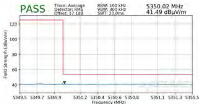
Plot 7-412. Radiated Upper Band Edge Plot MIMO (Average – UNII Band 2A – 484 Tones)
