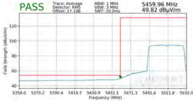
Plot 7-393. Radiated Lower Band Edge Plot SISO ANT2 (Average – UNII Band 2C – 484 Tones)
