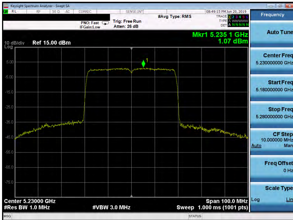
Plot 7-248. Power Spectral Density Plot MIMO ANT1 (40MHz BW 802.11ax – Full Tones (UNII Band 1) – Ch. 46)
