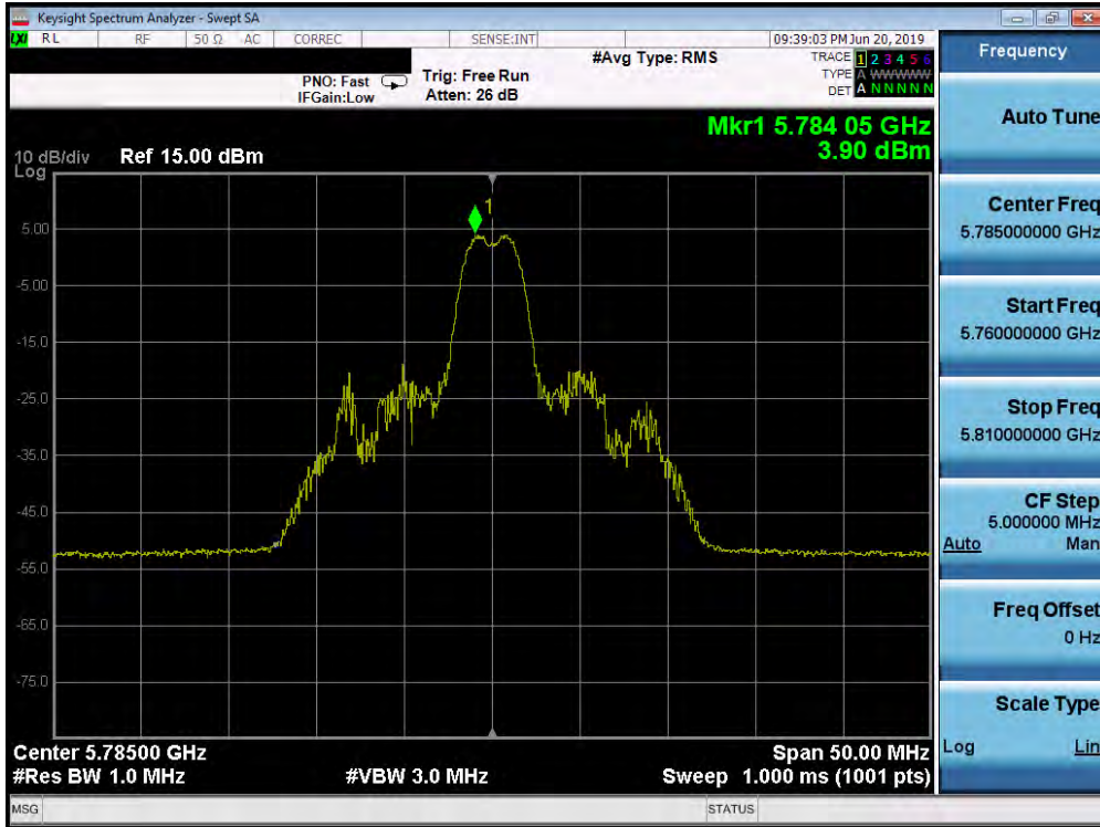
Plot 7-293. Power Spectral Density Plot MIMO ANT2 (20MHz BW 802.11ax – 26 Tones (UNII Band 3) – Ch. 157)
