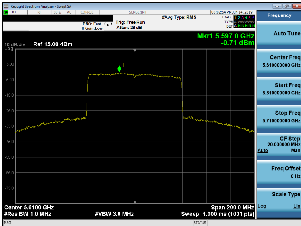
Plot 7-209. Power Spectral Density Plot SISO ANT2 (80MHz BW 802.11ax – Full Tones (UNII Band 2C) – Ch. 122)
