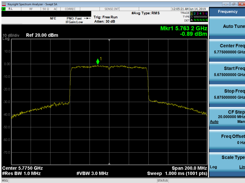
Plot 7-162. Power Spectral Density Plot SISO ANT1 (80MHz BW 802.11ax – Full Tones (UNII Band 3) – Ch. 155)
