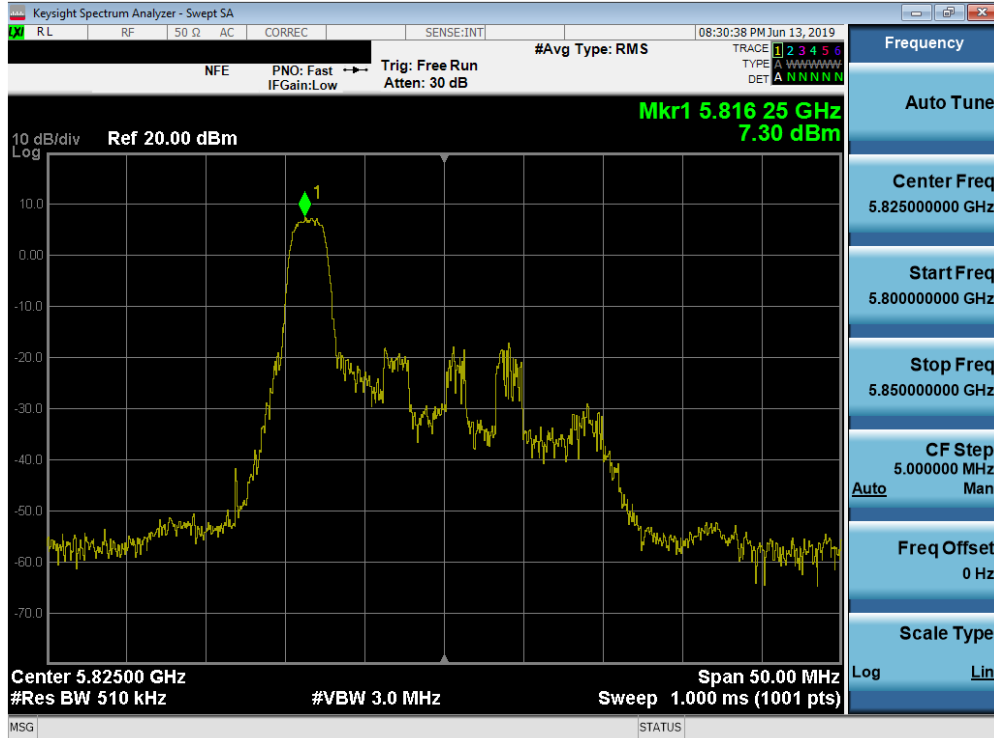
Plot 7-132. Power Spectral Density Plot SISO ANT1 (20 MHz BW 802.11ax – 26 Tones (UNII Band 3) – Ch. 165)
