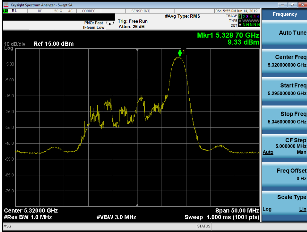
Plot 7-171. Power Spectral Density Plot SISO ANT2 (20MHz BW 802.11ax – 26 Tones (UNII Band 2A) – Ch. 64)
