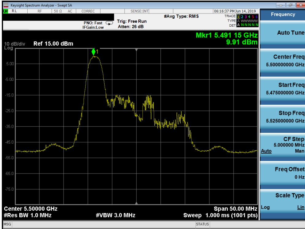
Plot 7-175. Power Spectral Density Plot SISO ANT2 (20MHz BW 802.11ax – 26 Tones (UNII Band 2C) – Ch. 100)
