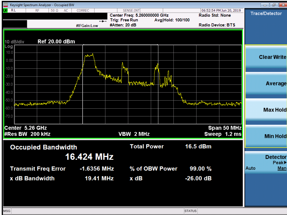
Plot 7-7. 26dB Bandwidth Plot SISO ANT1 (20MHz BW 802.11ax – 26 Tones (UNII Band 2A) – Ch. 52)
