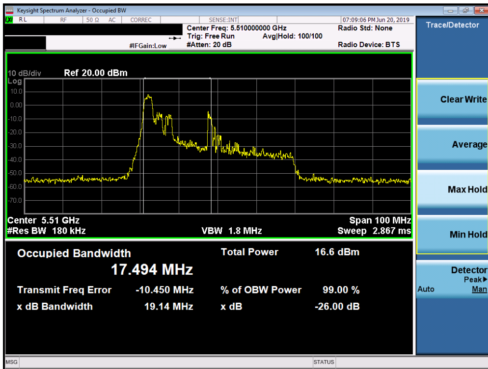
Plot 7-16. 26dB Bandwidth Plot SISO ANT1 (40MHz BW 802.11ax – 26 Tones (UNII Band 2C) – Ch. 102)
