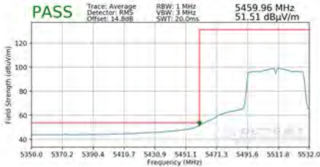
Plot 7-297. Radiated Lower Band Edge Plot SISO ANT1 (Average – UNII Band 2C)
