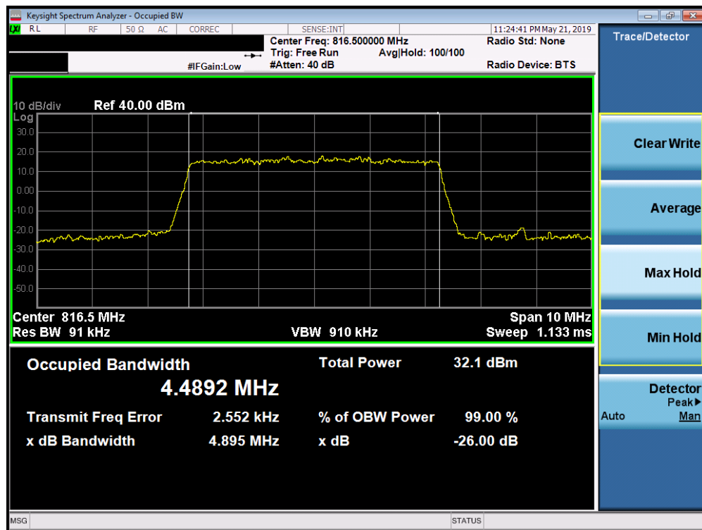
Plot 7-12. Occupied Bandwidth Plot (LTE Band 26, 5MHz 16-QAM – RB Size 25– Low Channel)
