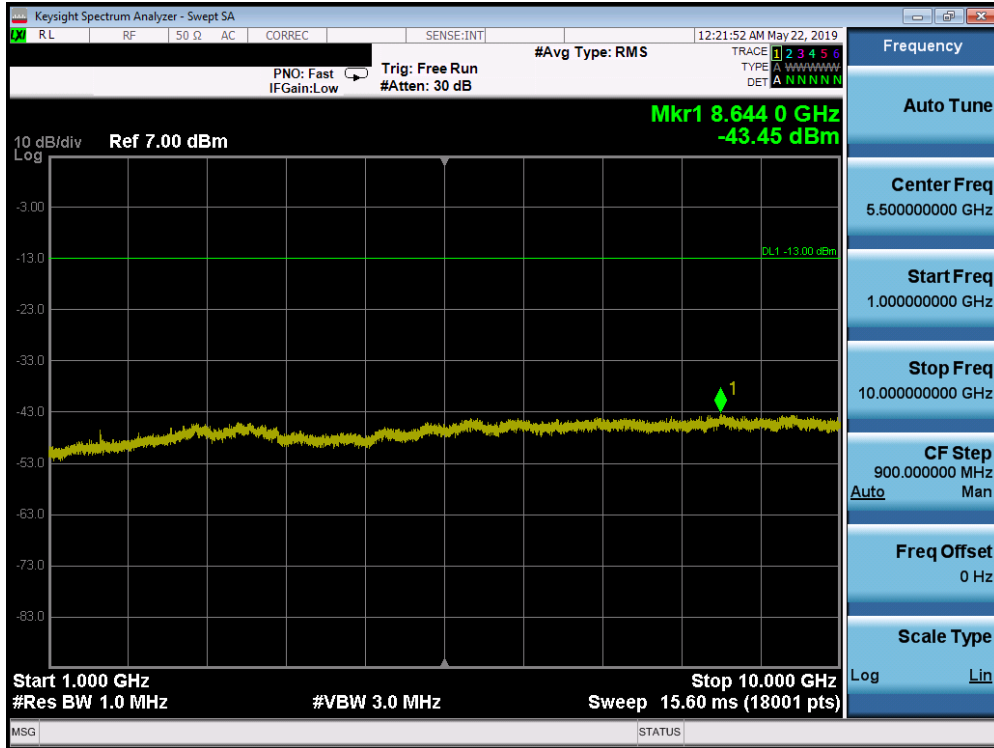
Plot 7-51. Conducted Spurious Plot (LTE Band 14, 5.0 MHz QPSK – RB Size 1, RB Offset 0 – High Channel)
