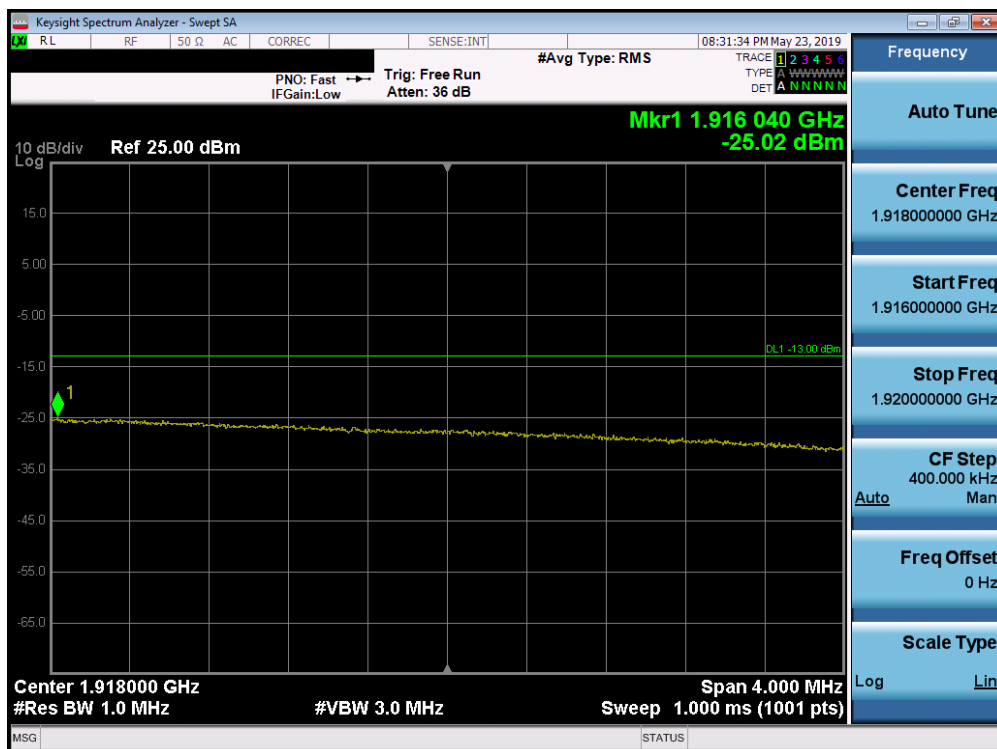
Plot 7-344. Upper Extended Band Edge Plot (Band 25 - 15.0MHz QPSK - Full RB Configuration)
