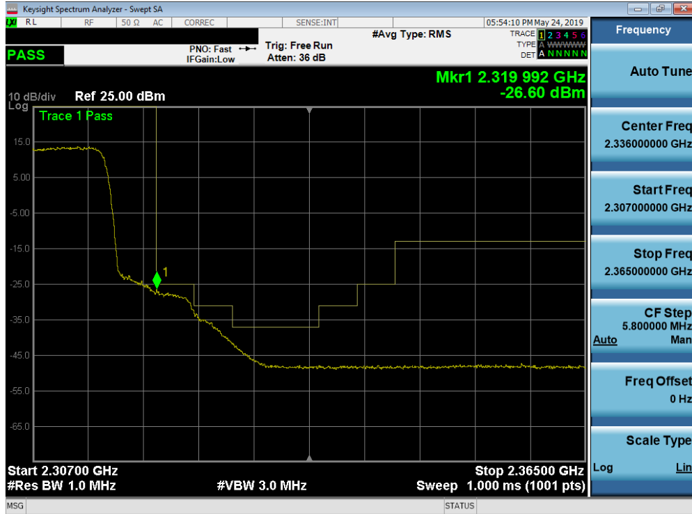
Plot 7-359. Upper Extended Band Edge Plot (Band 30 - 10.0MHz QPSK - Full RB Configuration)
