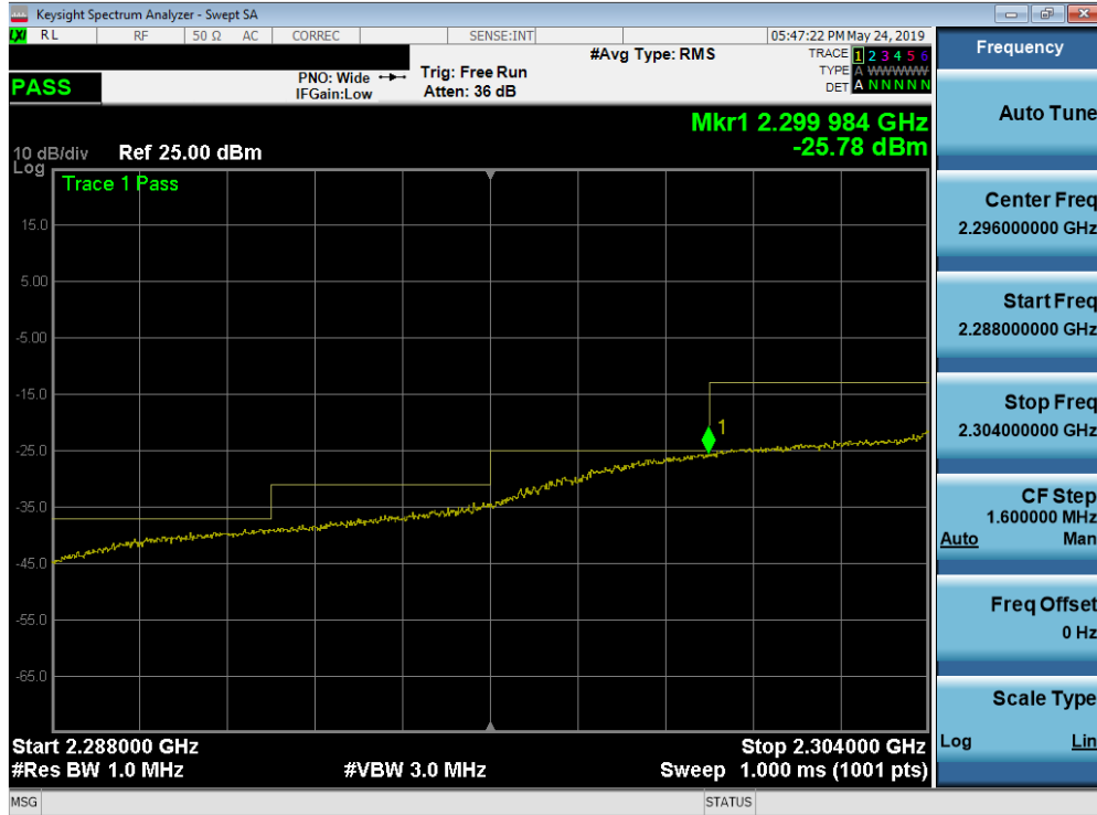
Plot 7-357. Lower Extended Band Edge Plot (Band 30 - 10.0MHz QPSK - Full RB Configuration)
