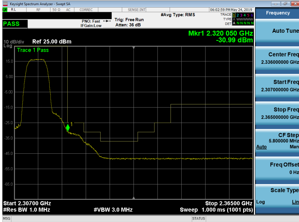
Plot 7-355. Upper Extended Band Edge Plot (Band 30 - 5.0MHz QPSK - Full RB Configuration)
