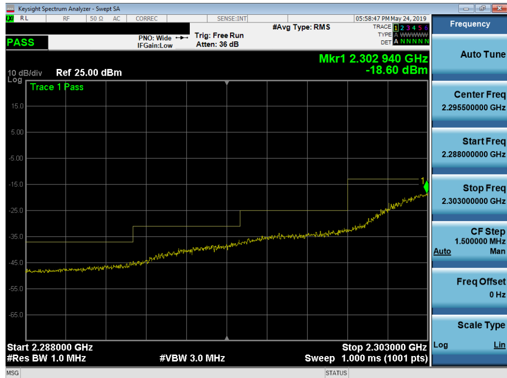
Plot 7-352. Lower Extended Band Edge Plot 2288-2303 MHz (Band 30 - 5.0MHz QPSK - Full RB Configuration)
