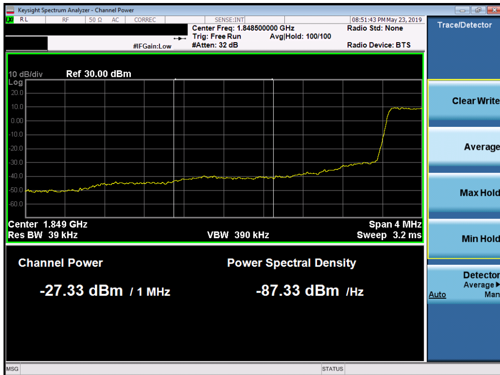
Plot 7-316. Lower Extended Band Edge Plot (Band 25/2 - 1.4MHz QPSK - Full RB Configuration)
