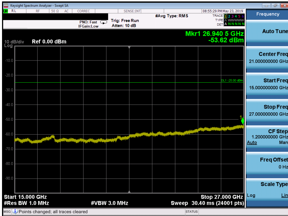
Plot 7-224. Conducted Spurious Plot (Band 7 - 20.0MHz QPSK - RB Size 1, RB Offset 0 - Low Channel)
