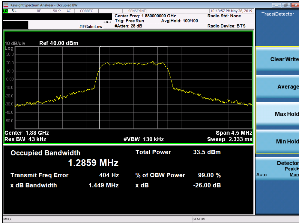
Plot 7-6. Occupied Bandwidth Plot (PCS CDMA Mode)
