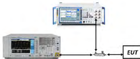
Figure 7-3. Test Instrument & Measurement Setup
