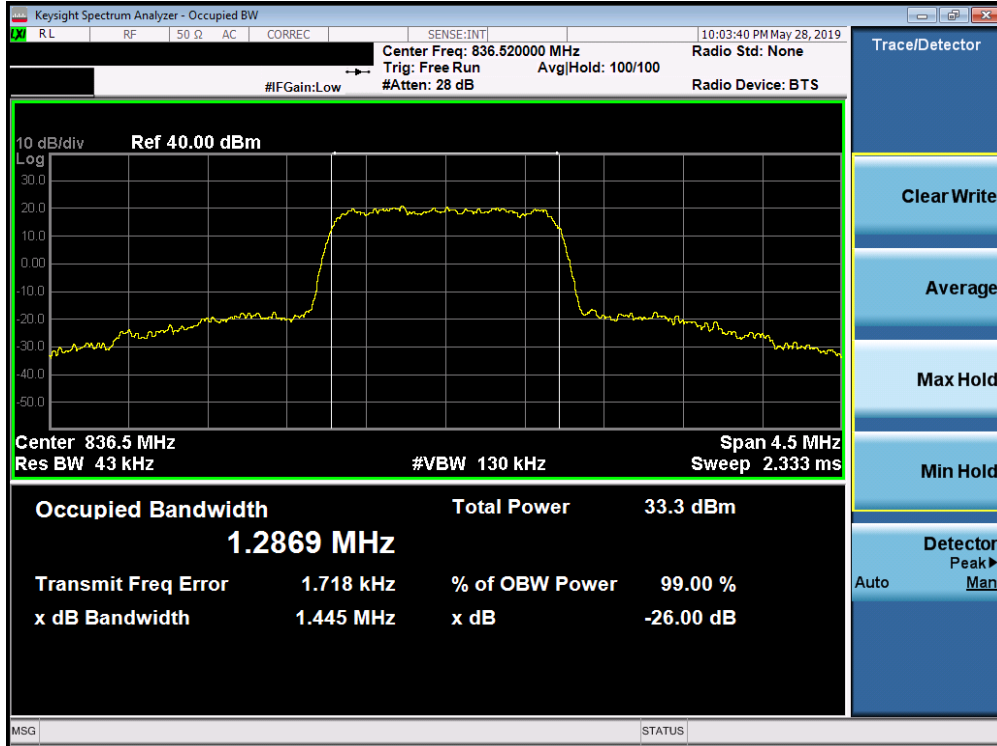
Plot 7-5. Occupied Bandwidth Plot (Cellular CDMA Mode)
