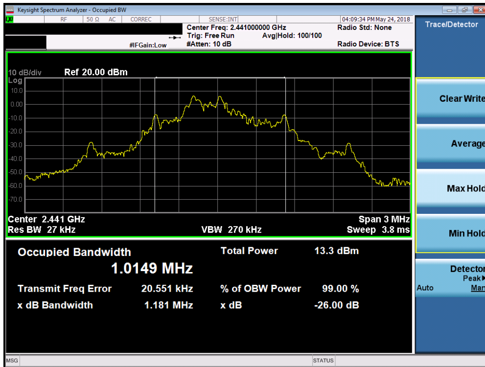
Plot 7-1. Occupied Bandwidth Plot (ANT+ – Ch. 39)
