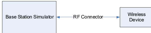
Figure 9-1 Power Measurement Setup
