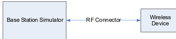
Figure 9-4 Power Measurement Setup
