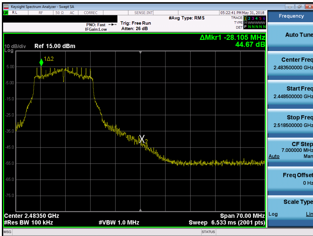
Plot 7-46. Band Edge Plot SISO ANT2 (802.11g - Ch. 11)
