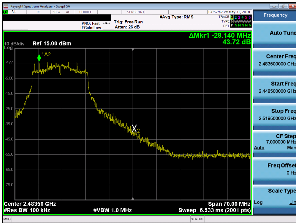
Plot 7-40. Band Edge Plot SISO ANT1 (802.11g - Ch. 11)
