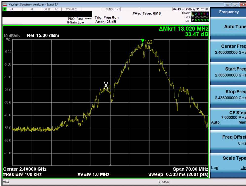
Plot 7-37. Band Edge Plot SISO ANT1 (802.11b – Ch. 1)
