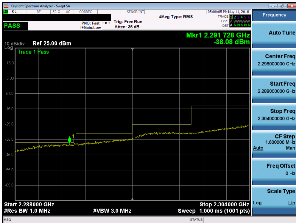
Plot 7-347. Lower Extended Band Edge Plot (Band 30 - 10.0MHz QPSK - Full RB Configuration)
