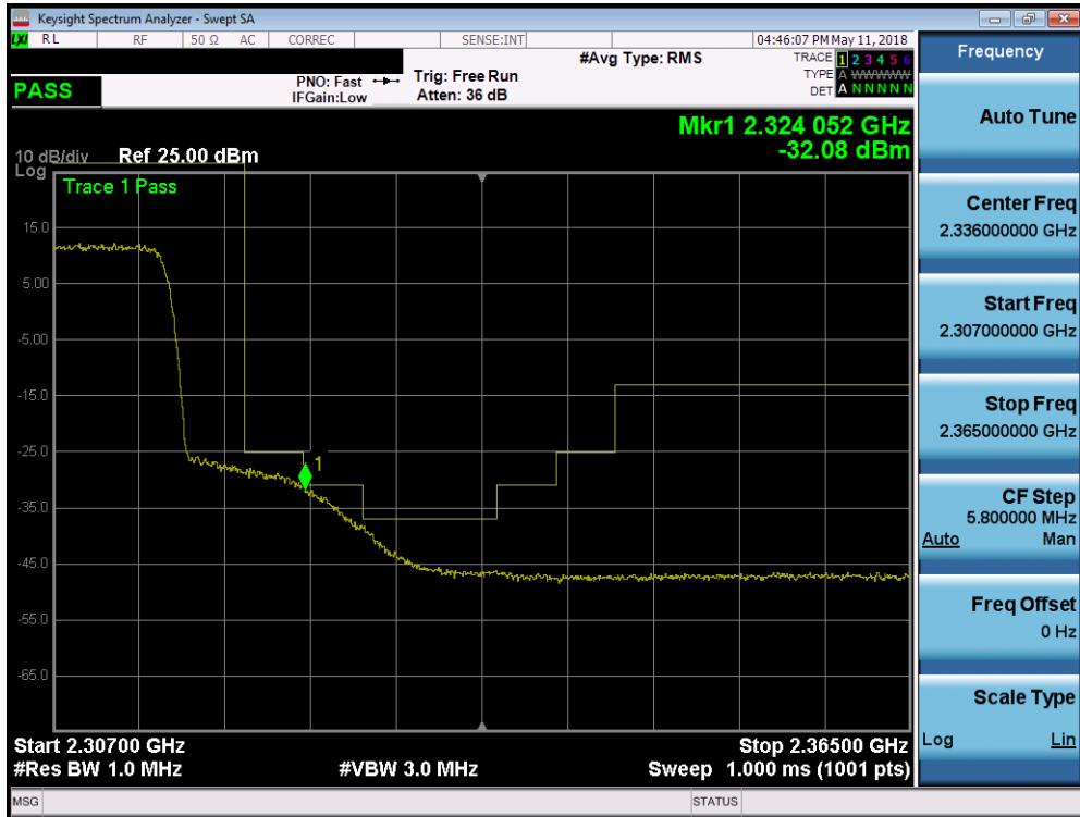
Plot 7-357. Upper Extended Band Edge Plot (Band 30 - 10.0MHz QPSK - Full RB Configuration)
