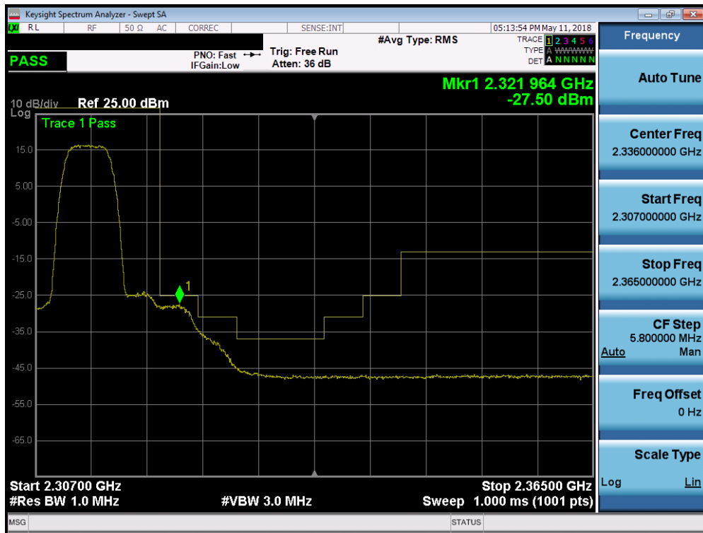
Plot 7-345. Upper Extended Band Edge Plot (Band 30 - 5.0MHz QPSK - Full RB Configuration)
