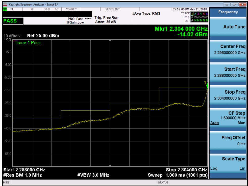
Plot 7-343. Lower Extended Band Edge Plot (Band 30 - 5.0MHz QPSK - Full RB Configuration)
