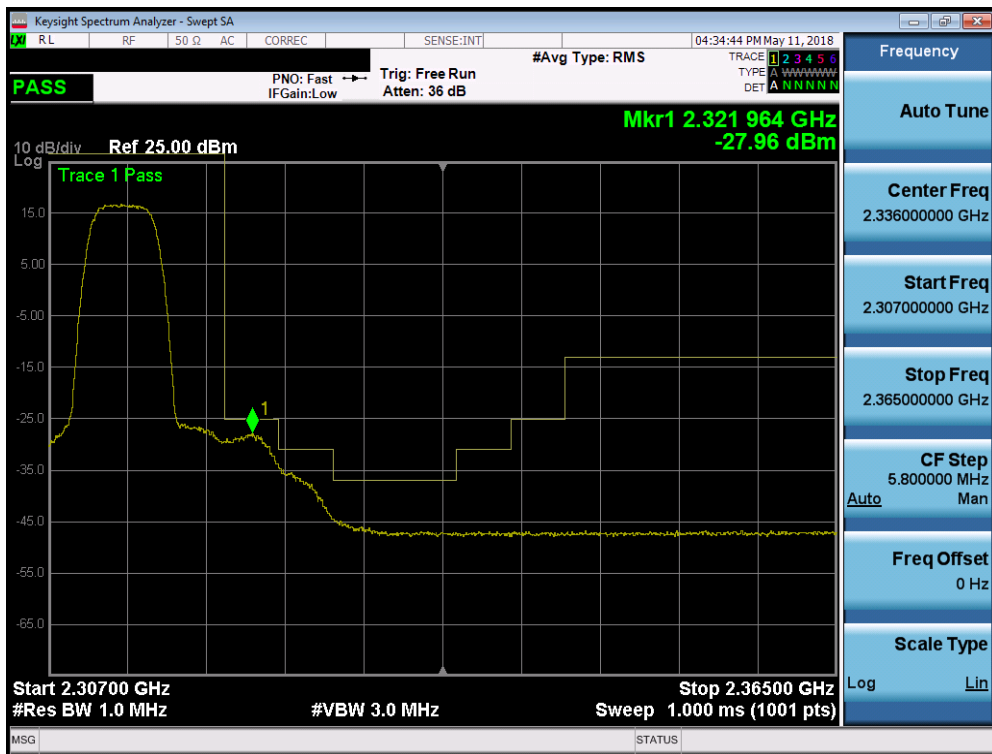
Plot 7-353. Upper Extended Band Edge Plot (Band 30 - 5.0MHz QPSK - Full RB Configuration)
