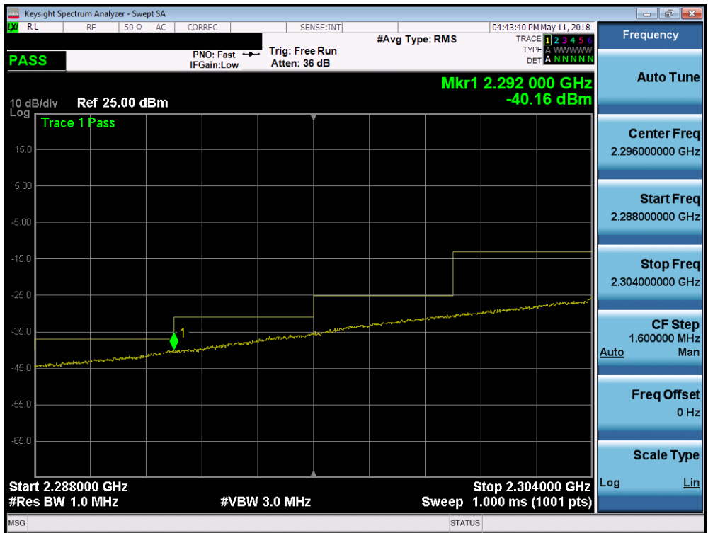
Plot 7-355. Lower Extended Band Edge Plot (Band 30 - 10.0MHz QPSK - Full RB Configuration)
