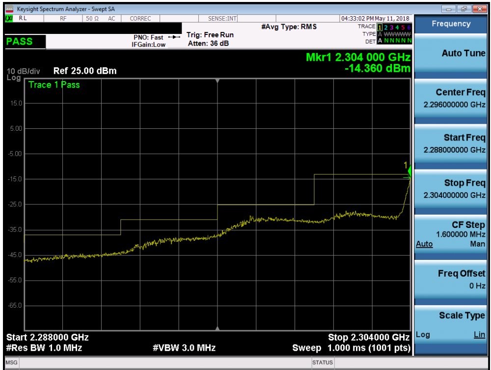
Plot 7-351. Lower Extended Band Edge Plot (Band 30 - 5.0MHz QPSK - Full RB Configuration)
