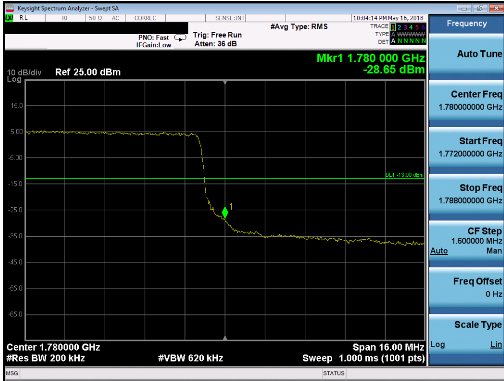
Plot 7-304. Upper Band Edge Plot (Band 66 - 20.0MHz QPSK - Full RB Configuration)
