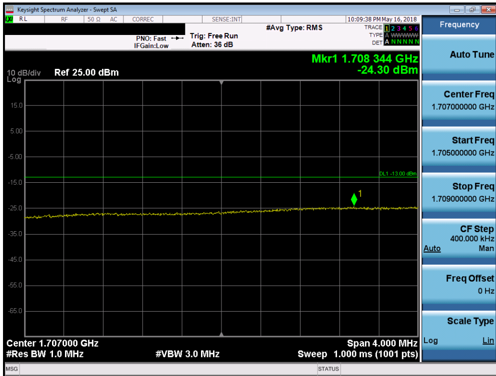
Plot 7-295. Lower Extended Band Edge Plot (Band 66/4 - 15.0MHz QPSK - Full RB Configuration)
