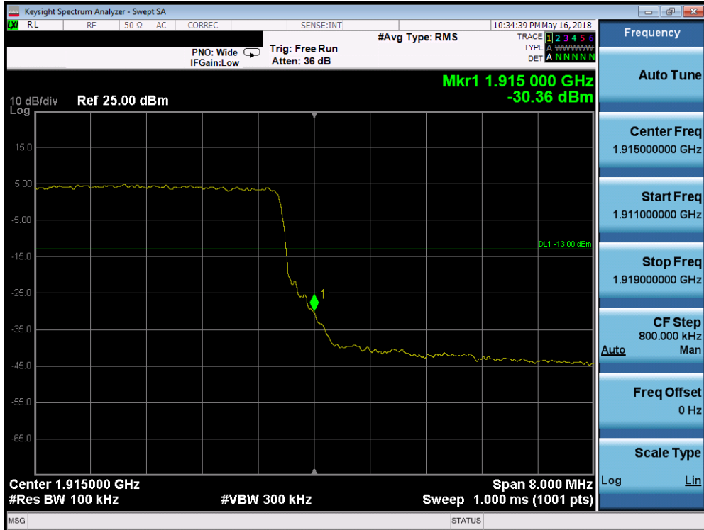
Plot 7-328. Upper Band Edge Plot (Band 25 - 10.0MHz QPSK - Full RB Configuration)
