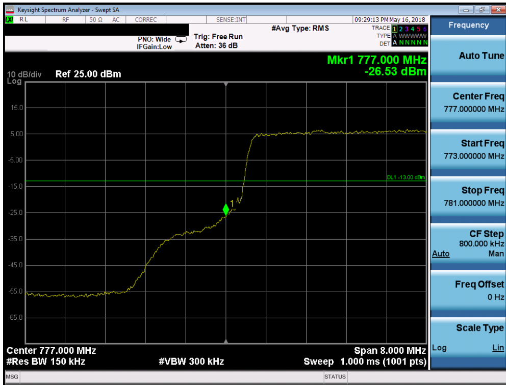
Plot 7-258. Lower Band Edge Plot (Band 13 - 10.0MHz QPSK - Full RB Configuration)
