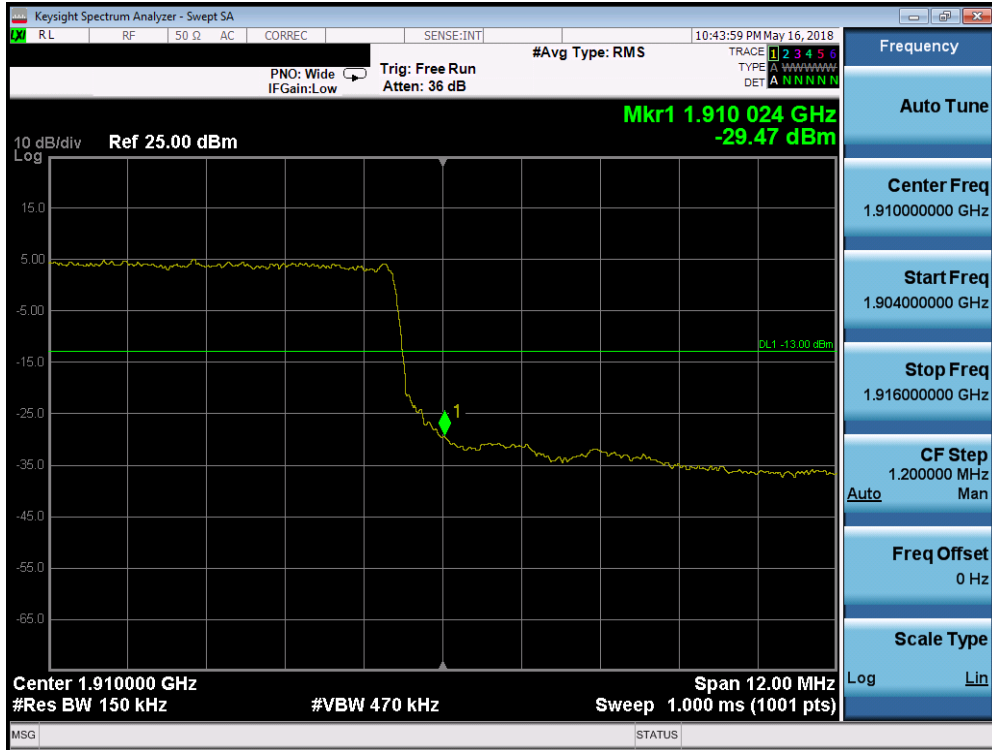
Plot 7-332. Upper Band Edge Plot (Band 2 - 15.0MHz QPSK - Full RB Configuration)
