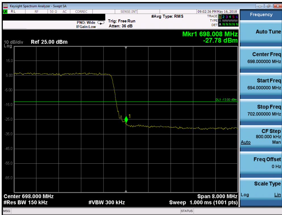
Plot 7-241. Upper Band Edge Plot (Band 71 - 10.0MHz QPSK - Full RB Configuration)
