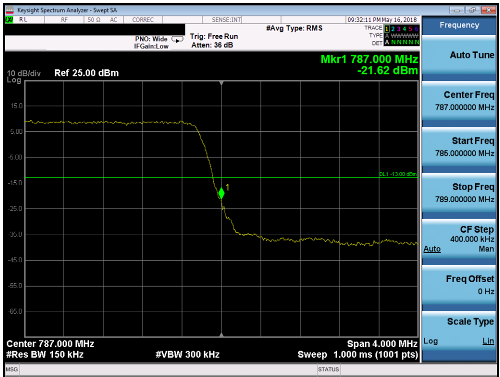
Plot 7-257. Upper Band Edge Plot (Band 13 - 5.0MHz QPSK - Full RB Configuration)
