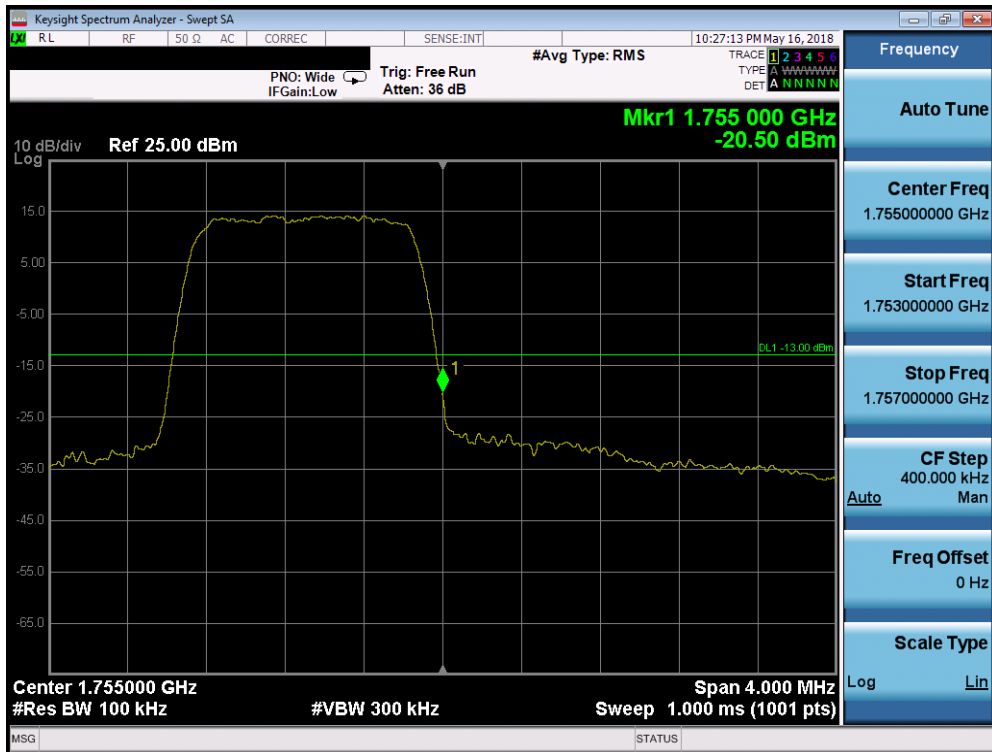
Plot 7-272. Upper Band Edge Plot (Band 4 - 1.4MHz QPSK - Full RB Configuration)
