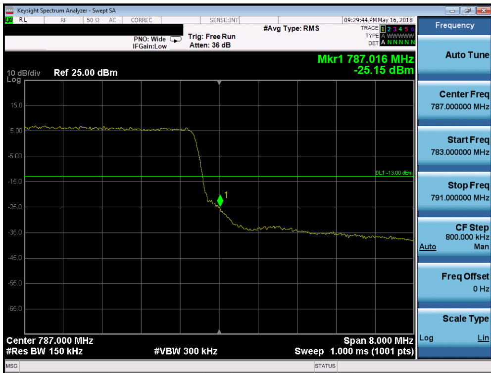
Plot 7-259. Upper Band Edge Plot (Band 13 - 10.0MHz QPSK - Full RB Configuration)
