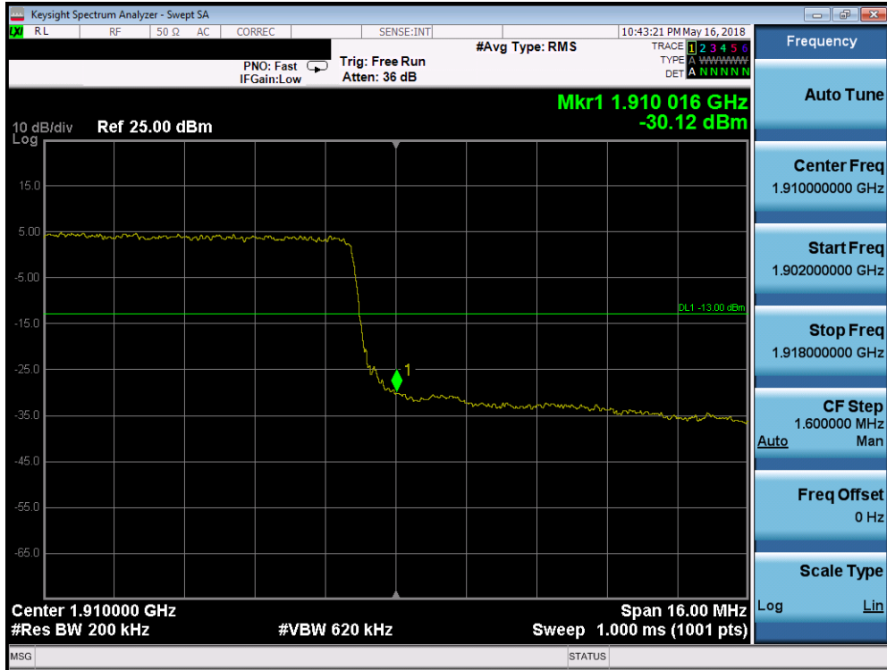
Plot 7-338. Upper Band Edge Plot (Band 2 - 20.0MHz QPSK - Full RB Configuration)
