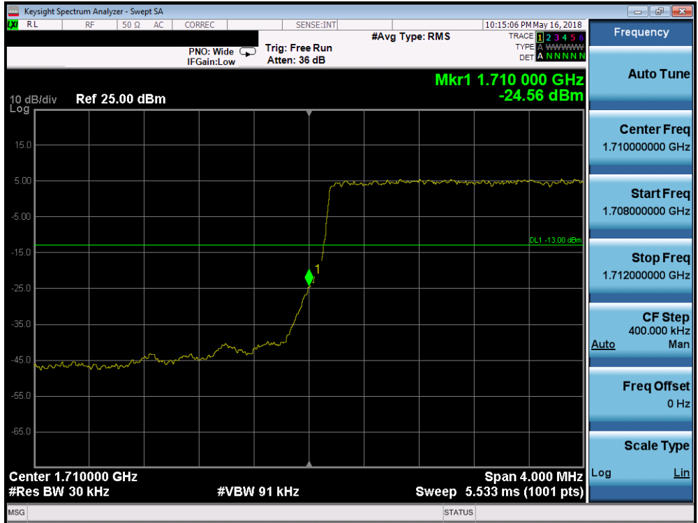
Plot 7-276. Lower Band Edge Plot (Band 66/4 - 3.0MHz QPSK - Full RB Configuration)
