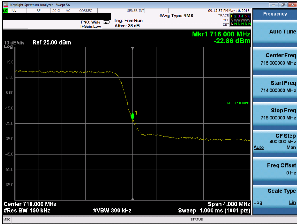
Plot 7-252. Upper Band Edge Plot (Band 12/17 - 5.0MHz QPSK - Full RB Configuration)
