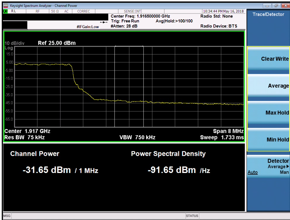
Plot 7-329. Upper Extended Band Edge Plot (Band 25 - 10.0MHz QPSK - Full RB Configuration)
