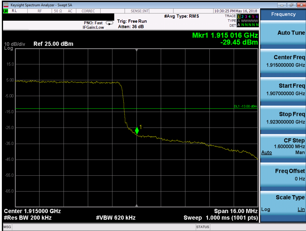
Plot 7-340. Upper Band Edge Plot (Band 25 - 20.0MHz QPSK - Full RB Configuration)
