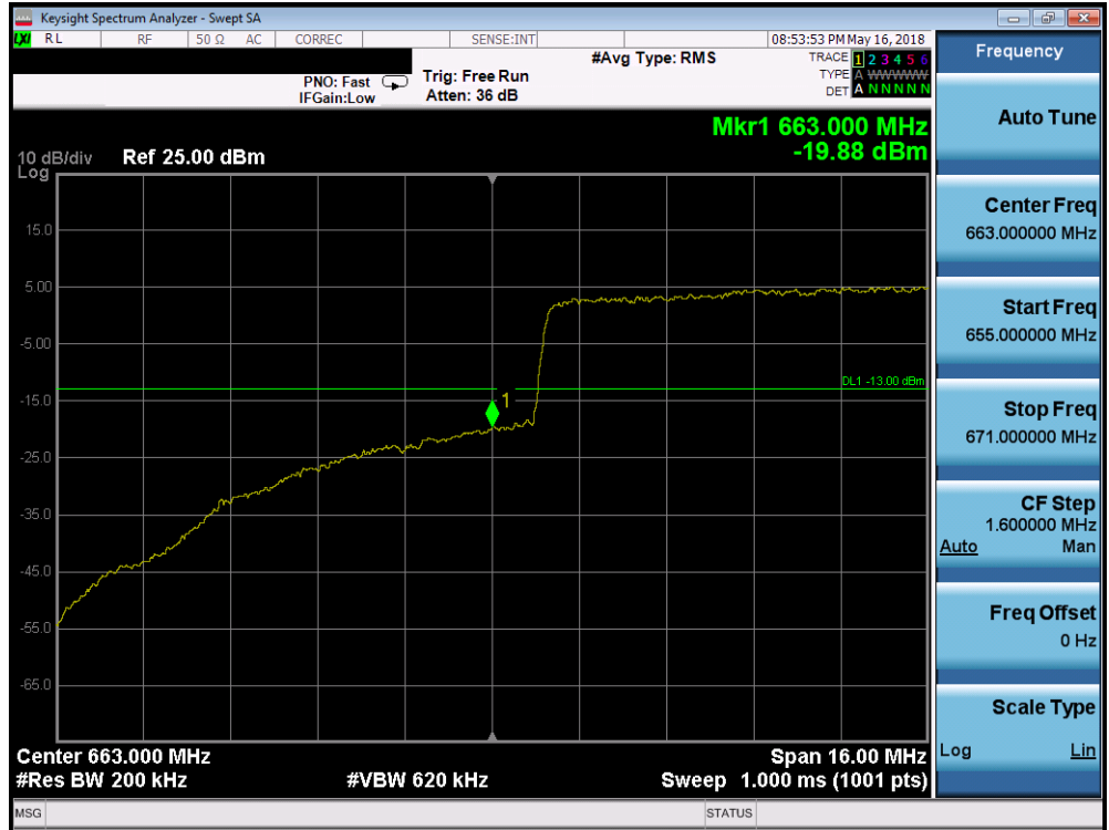
Plot 7-244. Lower Band Edge Plot (Band 71 - 20.0MHz QPSK - Full RB Configuration)
