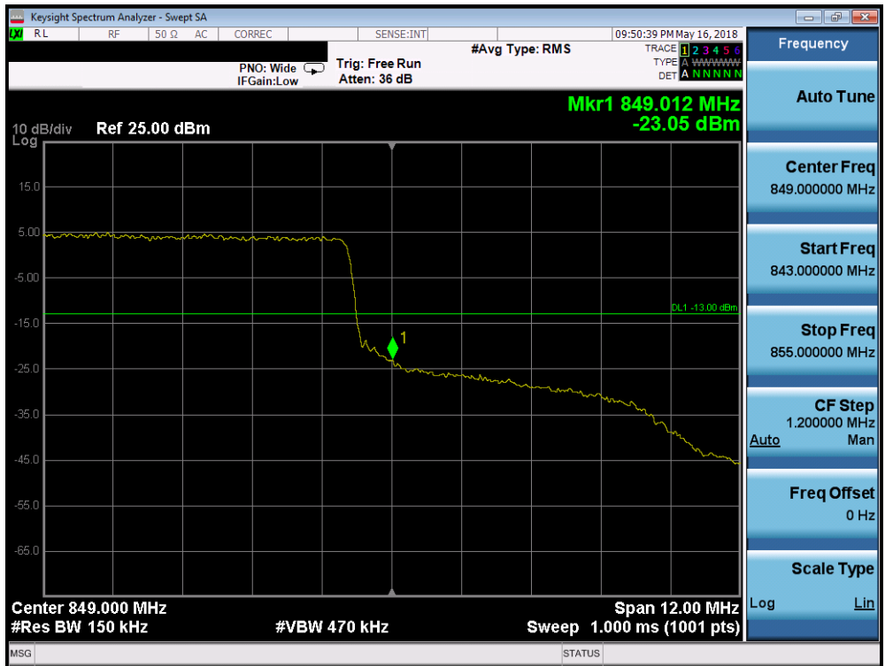
Plot 7-269. Upper Band Edge Plot (Band 26 - 15.0MHz QPSK - Full RB Configuration)
