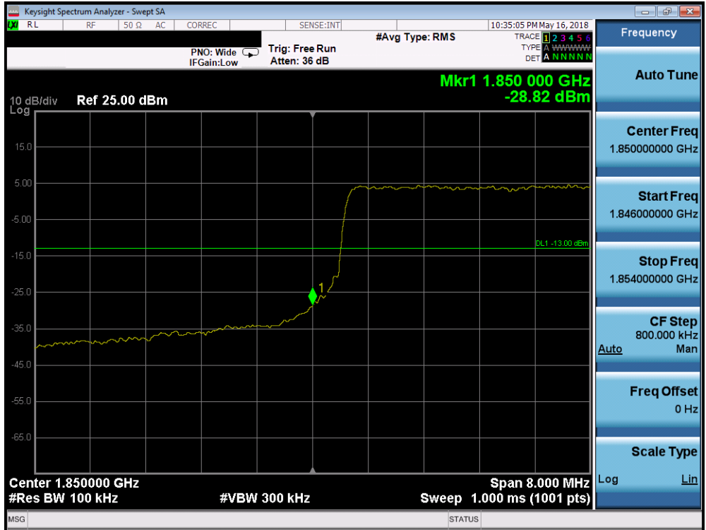
Plot 7-324. Lower Band Edge Plot (Band 25/2 - 10.0MHz QPSK - Full RB Configuration)
