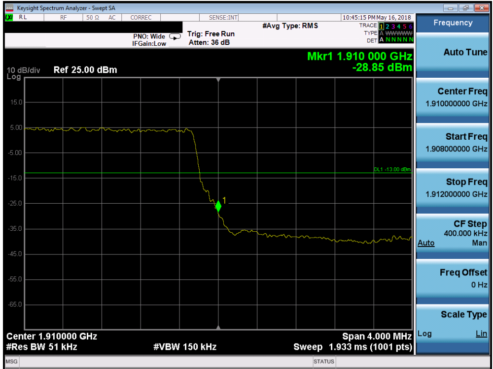
Plot 7-320. Upper Band Edge Plot (Band 2 - 5.0MHz QPSK - Full RB Configuration)
