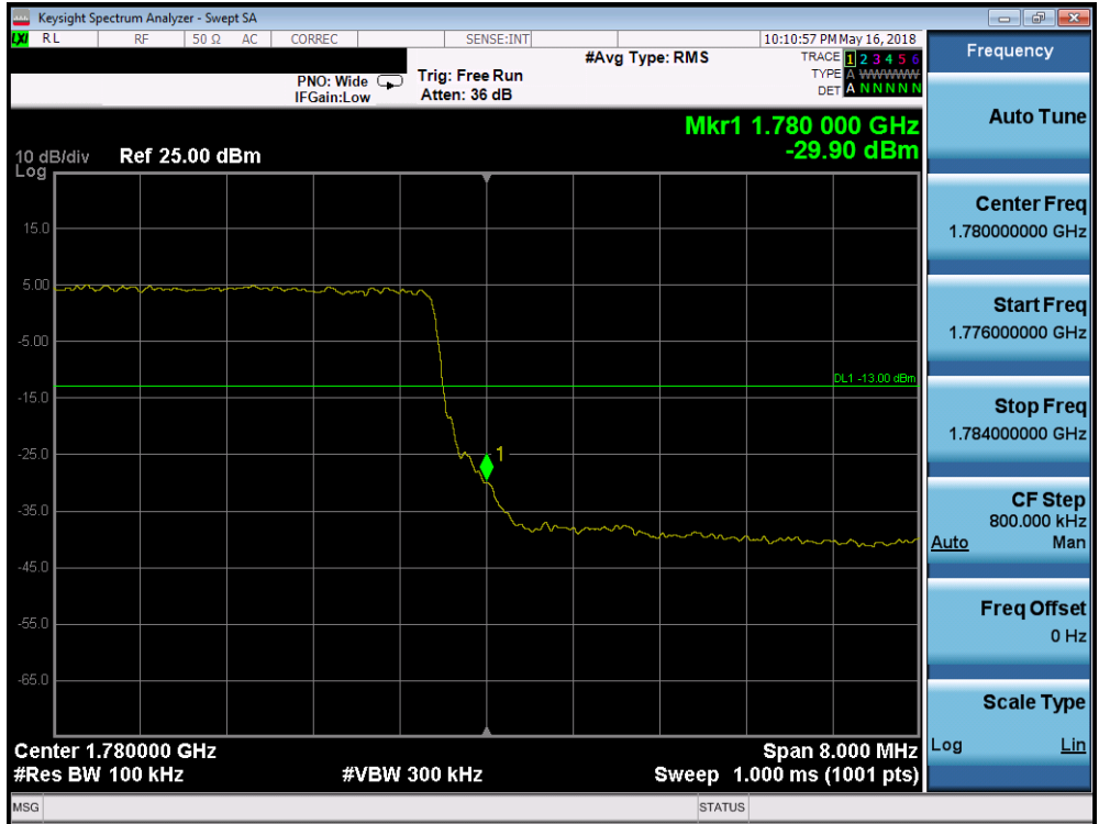
Plot 7-292. Upper Band Edge Plot (Band 66 - 10.0MHz QPSK - Full RB Configuration)
