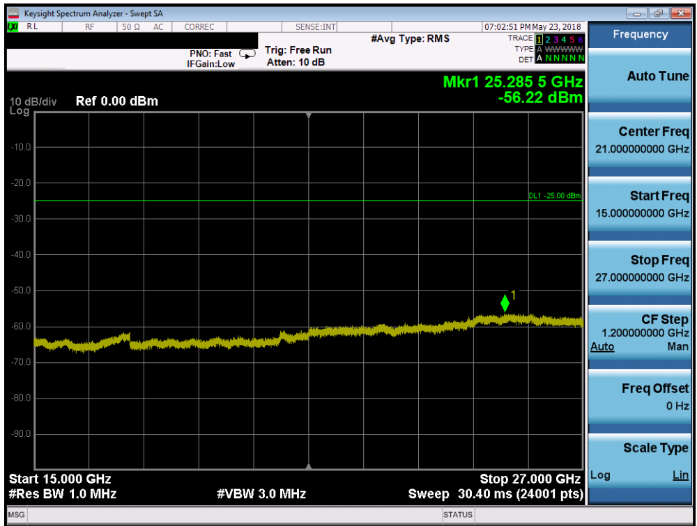
Plot 7-213. Conducted Spurious Plot (Band 7 - 15.0MHz QPSK - RB Size 1, RB Offset 0 - Low Channel)
