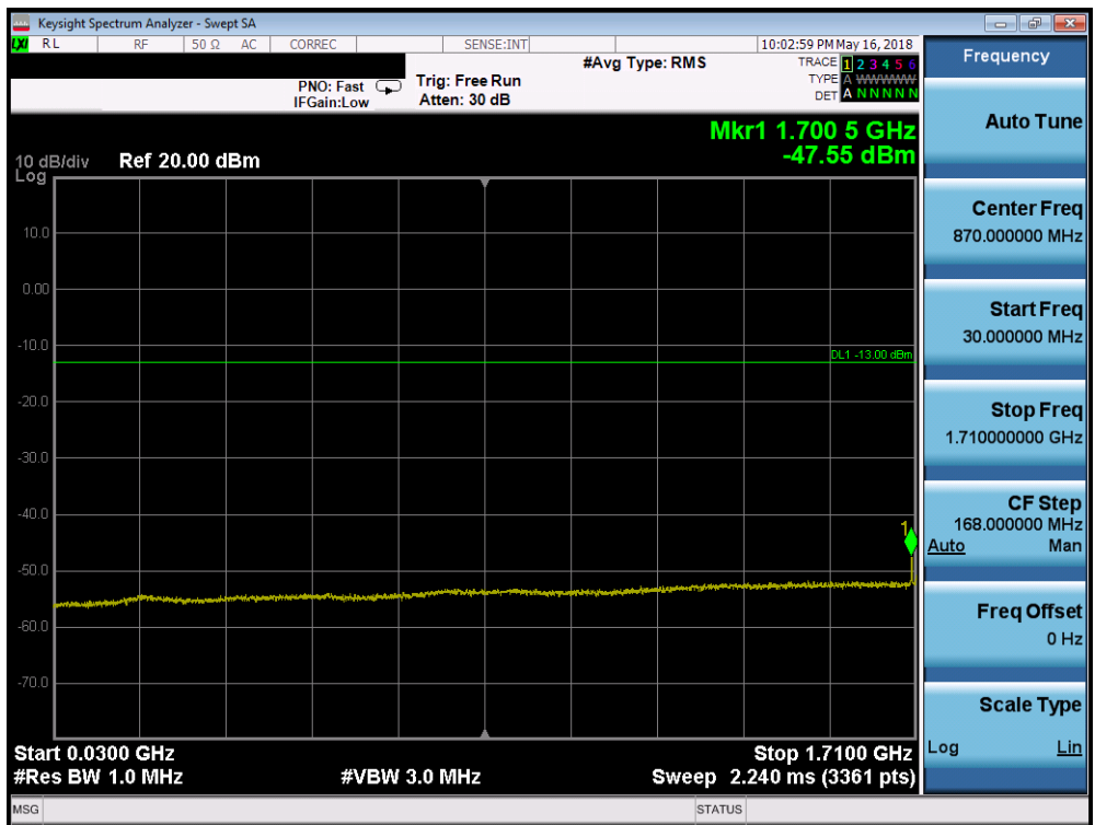
Plot 7-175. Conducted Spurious Plot (Band 66/4 - 20.0MHz QPSK - RB Size 1, RB Offset 0 - Mid Channel)
