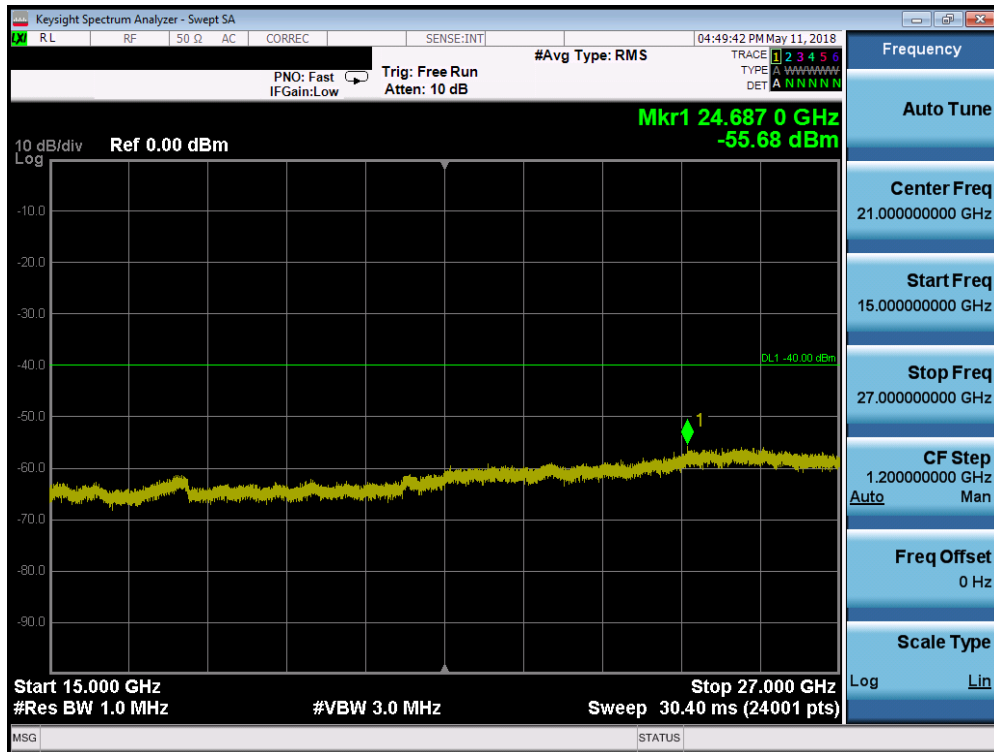
Plot 7-192. Conducted Spurious Plot (Band 30 - 10.0MHz QPSK - RB Size 1, RB Offset 0 - Mid Channel)
