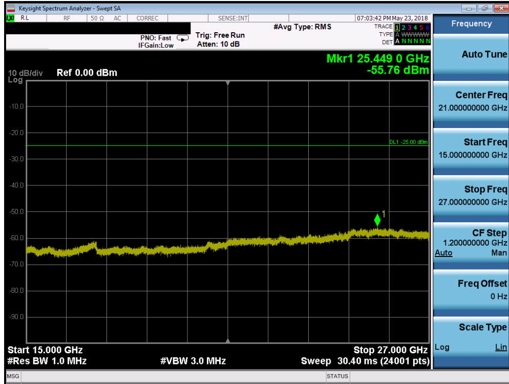
Plot 7-219. Conducted Spurious Plot (Band 7 - 15.0MHz QPSK - RB Size 1, RB Offset 0 - High Channel)
