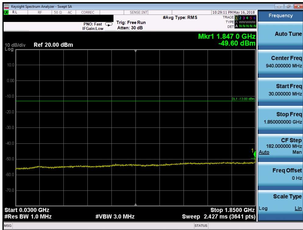
Plot 7-184. Conducted Spurious Plot (Band 25/2 - 20.0MHz QPSK - RB Size 1, RB Offset 0 - Mid Channel)
