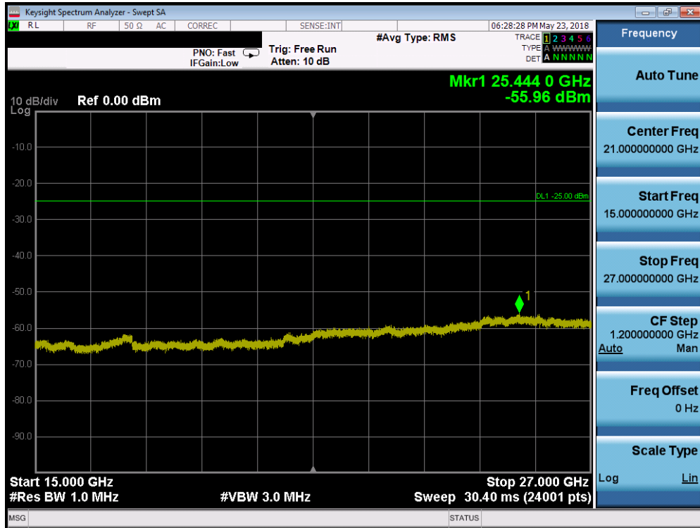
Plot 7-204. Conducted Spurious Plot (Band 7 - 15.0MHz QPSK - RB Size 1, RB Offset 0 - Low Channel)
