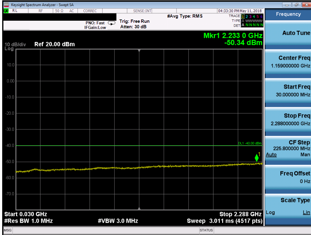
Plot 7-199. Conducted Spurious Plot (Band 30 - 5.0MHz QPSK - RB Size 1, RB Offset 0 - High Channel)
