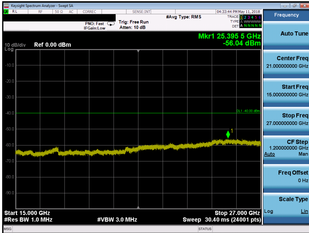
Plot 7-201. Conducted Spurious Plot (Band 30 - 5.0MHz QPSK - RB Size 1, RB Offset 0 - High Channel)
