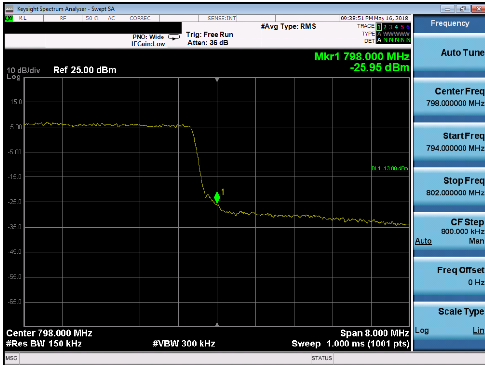
Plot 7-44. Upper Band Edge Plot (LTE Band 14 – 10MHz QPSK – Full RB Configuration)
