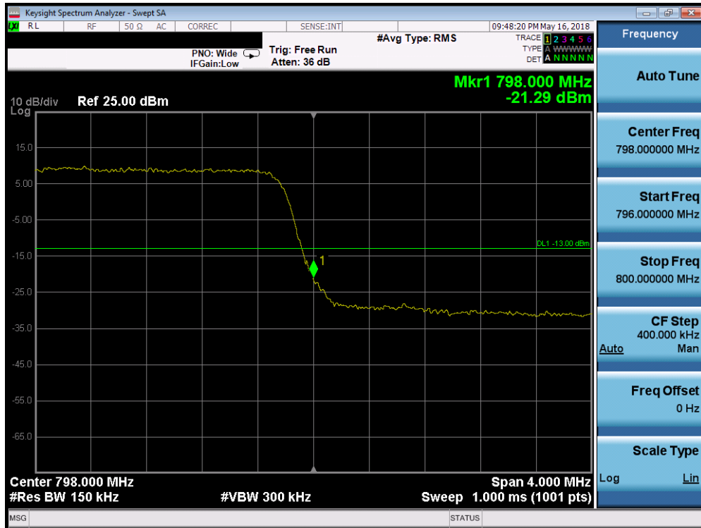
Plot 7-40. Upper Band Edge Plot (LTE Band 14 – 5MHz QPSK – Full RB Configuration)
