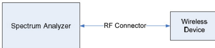
Figure 7-1. Test Instrument & Measurement Setup
