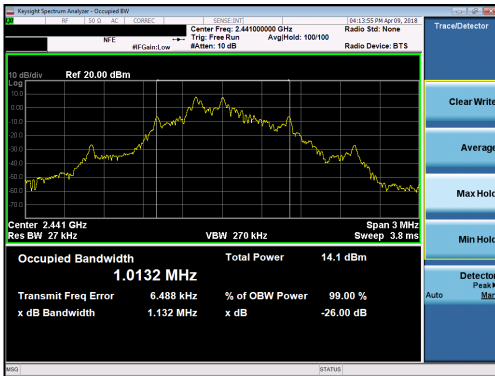
Plot 7-1. Occupied Bandwidth Plot (ANT+ – Ch. 39)
