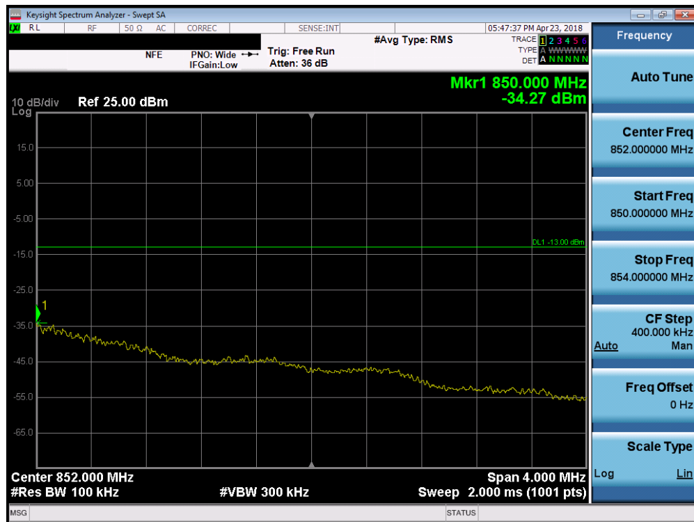
Plot 7-157. Upper Extended Band Edge Plot (Band 26/5 - 1.4MHz QPSK - Full RB Configuration)
