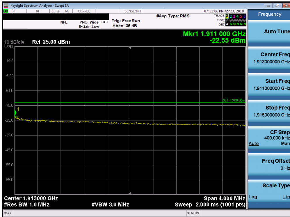
Plot 7-225. Upper Extended Band Edge Plot (Band 2 - 10.0MHz QPSK - Full RB Configuration)
