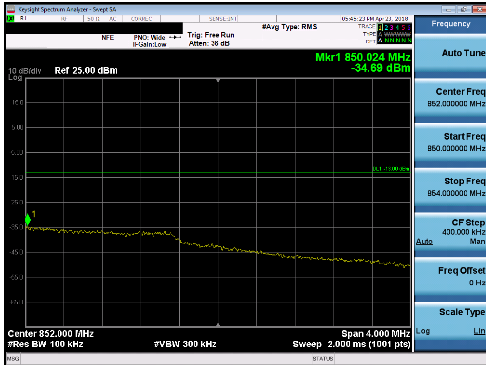
Plot 7-161. Upper Extended Band Edge Plot (Band 26/5 - 3.0MHz QPSK - Full RB Configuration)
