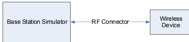
Figure 9-1 Power Measurement Setup
