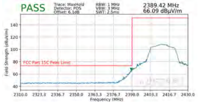
Plot 7-102. Radiated Restricted Lower Band Edge Measurement MIMO (Peak)
