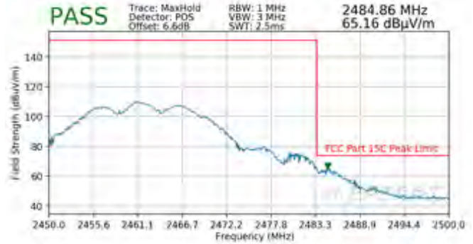
Plot 7-114. Radiated Restricted Upper Band Edge Measurement CDD (Peak)
