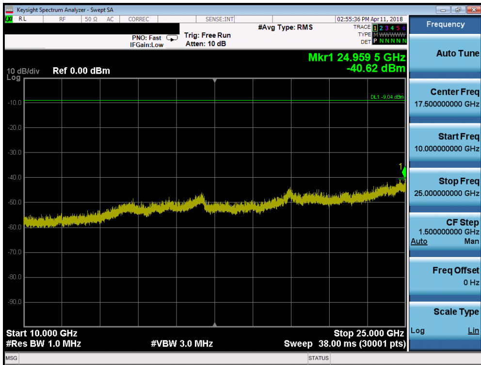
Plot 7-64. Conducted Spurious Plot SISO ANT1 (802.11b – Ch. 6)
