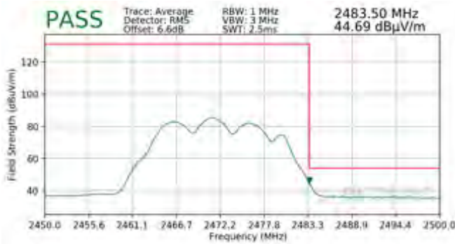
Plot 7-117. Radiated Restricted Upper Band Edge Measurement CDD (Average)
