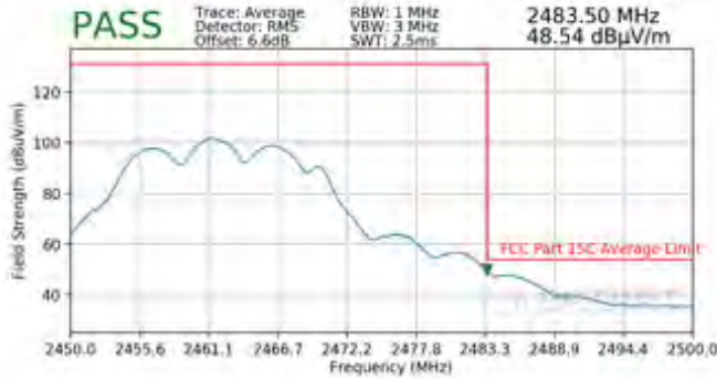
Plot 7-113. Radiated Restricted Upper Band Edge Measurement CDD (Average)
