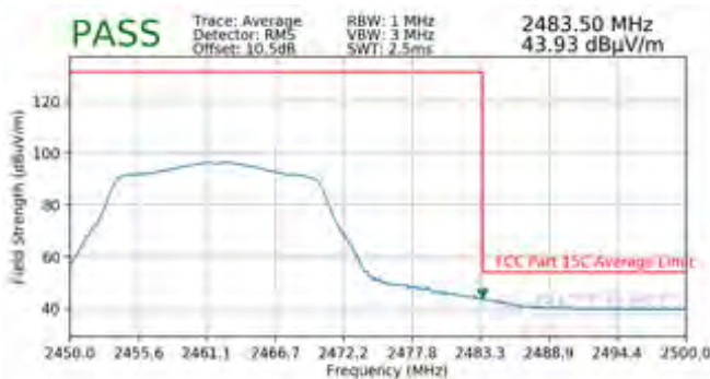
Plot 7-83. Radiated Restricted Upper Band Edge Measurement SISO ANT1 (Average)
