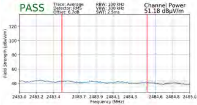
Plot 7-109. Radiated Restricted Band Edge Measurement MIMO with WCP (Average)
