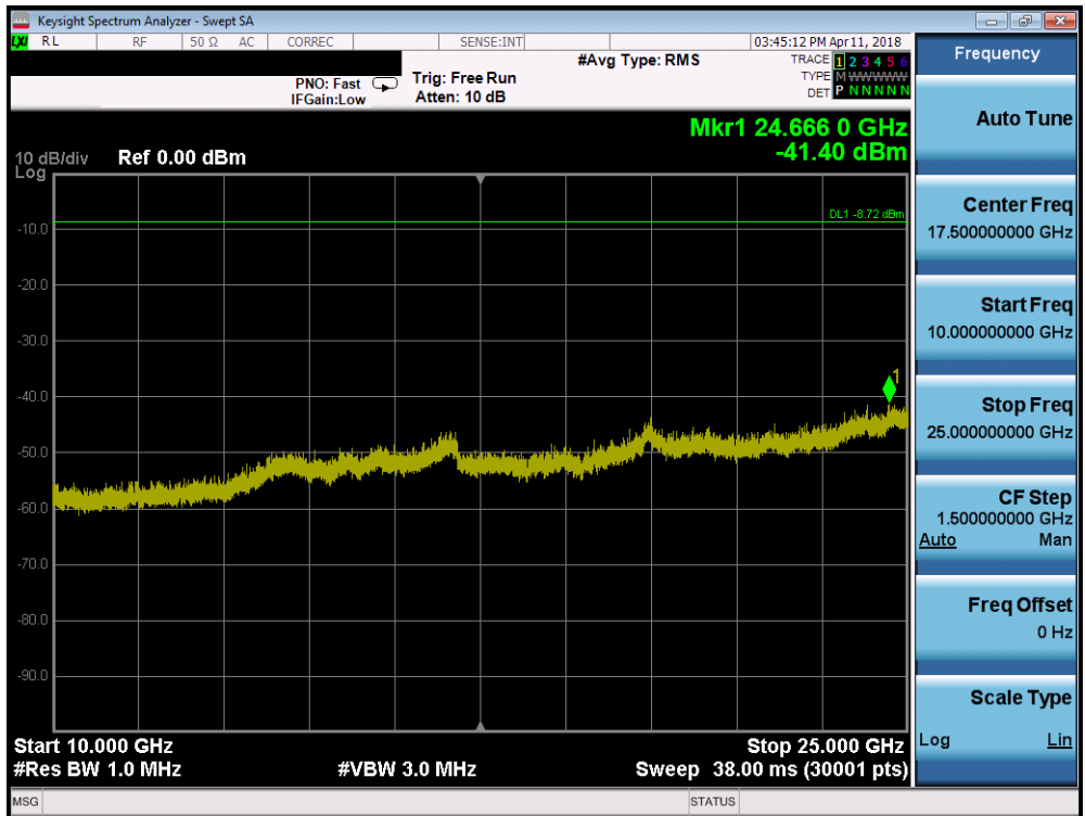
Plot 7-72. Conducted Spurious Plot SISO ANT2 (802.11b – Ch. 11)
