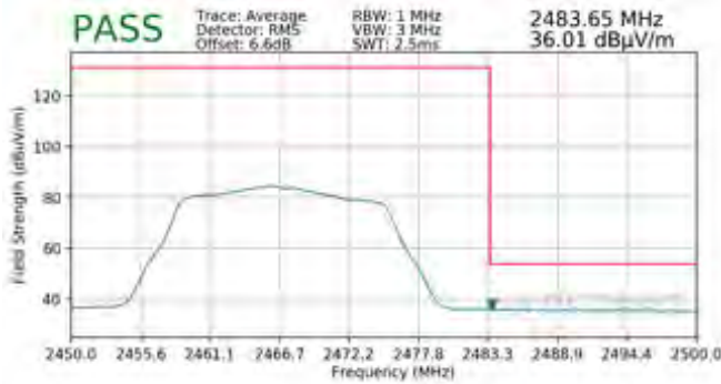
Plot 7-85. Radiated Restricted Upper Band Edge Measurement SISO ANT1 (Average)
