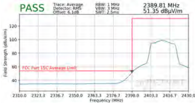
Plot 7-101. Radiated Restricted Lower Band Edge Measurement MIMO (Average)
