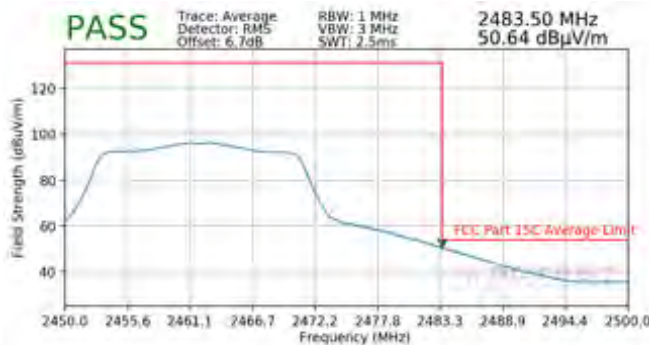
Plot 7-93. Radiated Restricted Upper Band Edge Measurement SISO ANT2 (Average)
