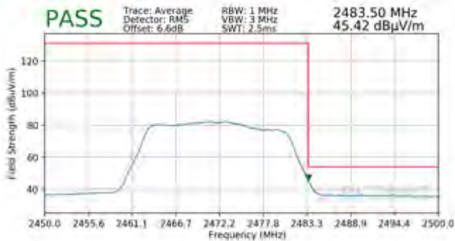
Plot 7-107. Radiated Restricted Upper Band Edge Measurement MIMO (Average)
