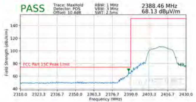
Plot 7-92. Radiated Restricted Lower Band Edge Measurement SISO ANT2 (Peak)
