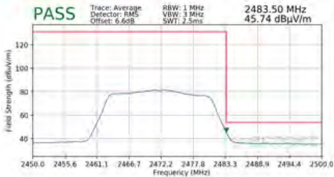
Plot 7-97. Radiated Restricted Upper Band Edge Measurement SISO ANT2 (Average)
