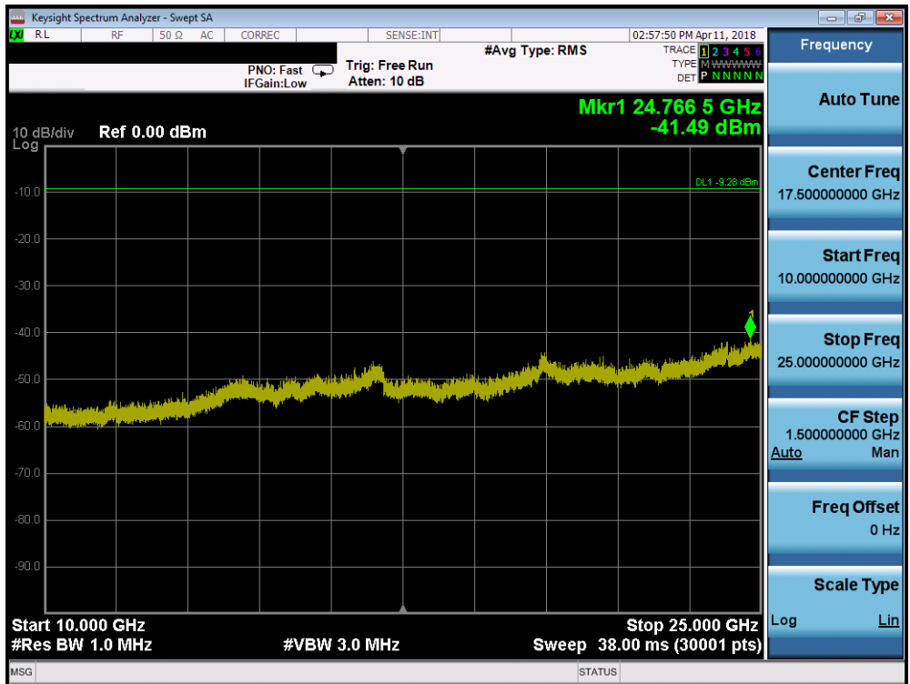
Plot 7-66. Conducted Spurious Plot SISO ANT1 (802.11b – Ch. 11)
