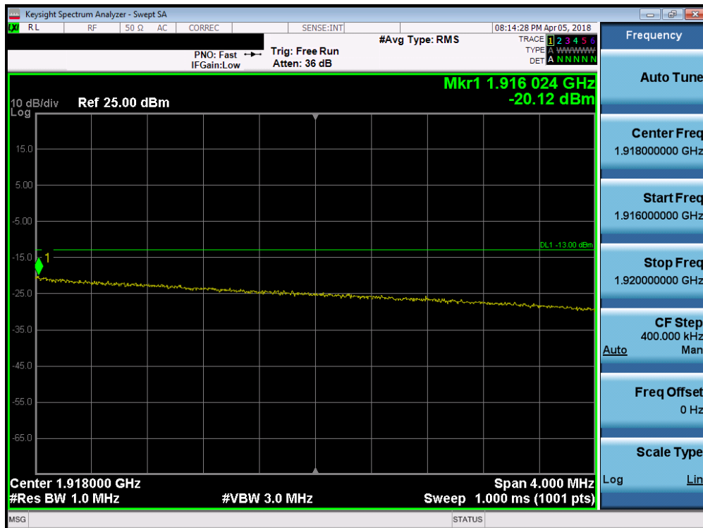
Plot 7-240. Upper Extended Band Edge Plot (Band 25 - 10.0MHz QPSK - Full RB Configuration)
