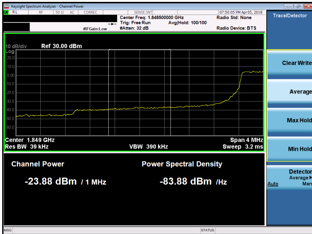
Plot 7-224. Lower Extended Band Edge Plot (Band 25/2 - 3.0MHz QPSK - Full RB Configuration)
