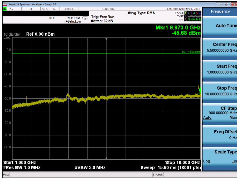
Plot 7-120. Conducted Spurious Plot (Band 26/5 - 3.0MHz QPSK - RB Size 1, RB Offset 0 - High Channel)
