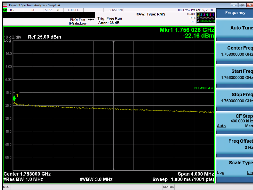
Plot 7-202. Upper Extended Band Edge Plot (Band 4 - 10.0MHz QPSK - Full RB Configuration)
