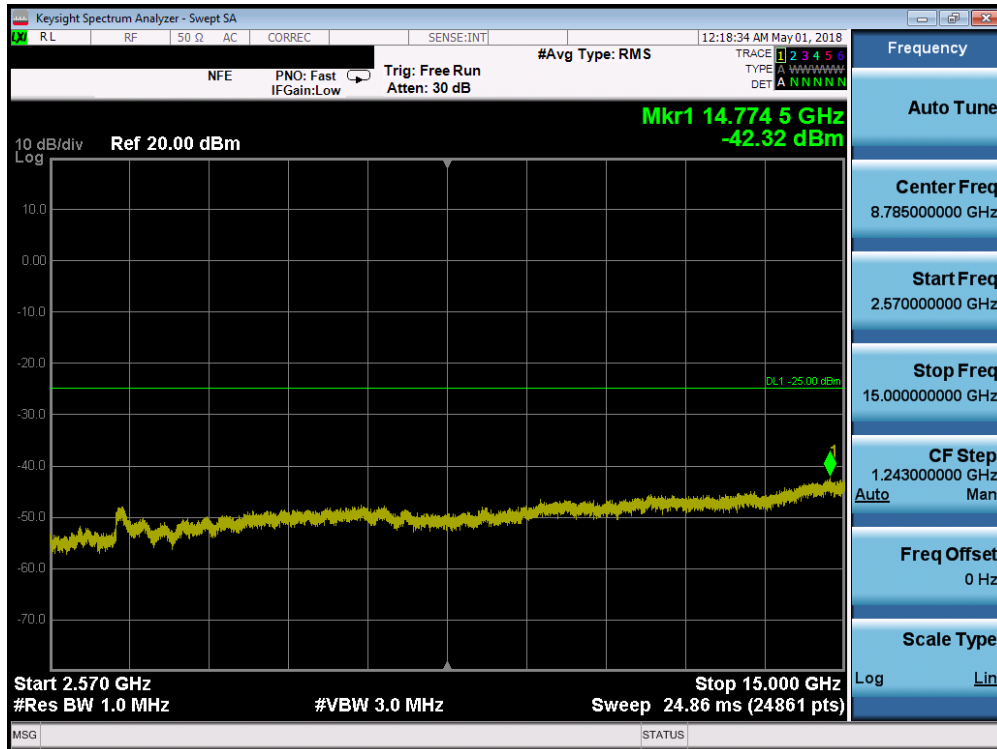
Plot 7-143. Conducted Spurious Plot (Band 7 - 20.0MHz QPSK - RB Size 1, RB Offset 0 - Mid Channel)
