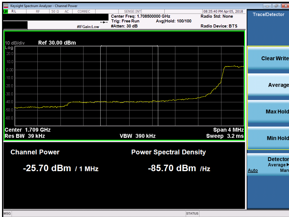
Plot 7-188. Lower Extended Band Edge Plot (Band 66/4 - 3.0MHz QPSK - Full RB Configuration)
