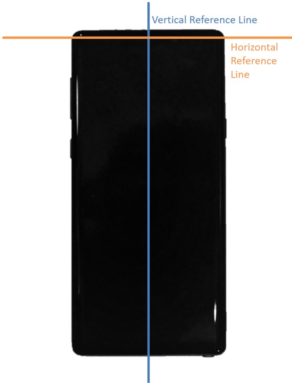
SAR Test Setup Photo 20 – Horizontal and Vertical Reference Lines
