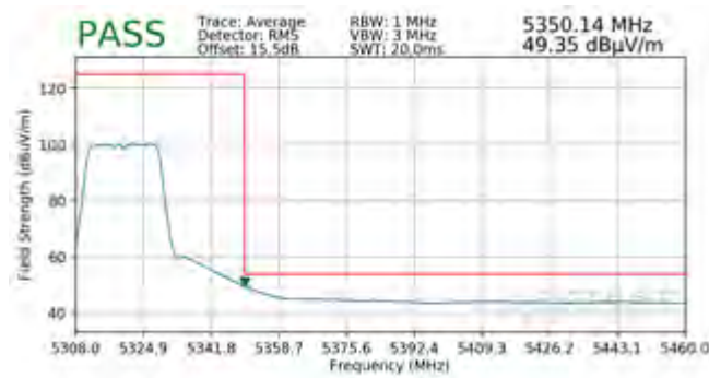
Plot 7-235. Radiated Band Edge Plot (Average – WCP)
