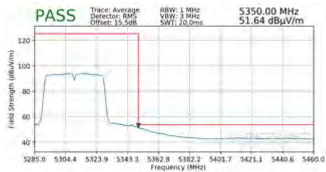
Plot 7-190. Radiated Band Edge Plot (Average – WCP)
