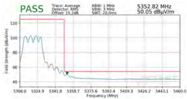
Plot 7-244. Radiated Band Edge Plot (Average – WCP)
