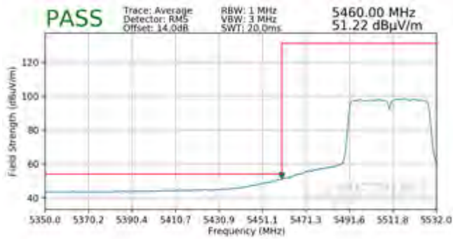
Plot 7-253. Radiated Band Edge Plot (Average – WCP)
