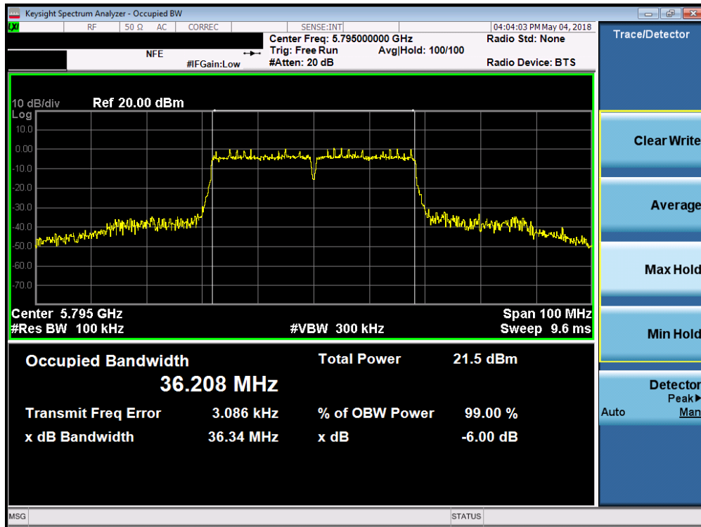
Plot 7-66. 6dB Bandwidth Plot (40MHz BW 802.11n (UNII Band 3) – Ch. 159)
