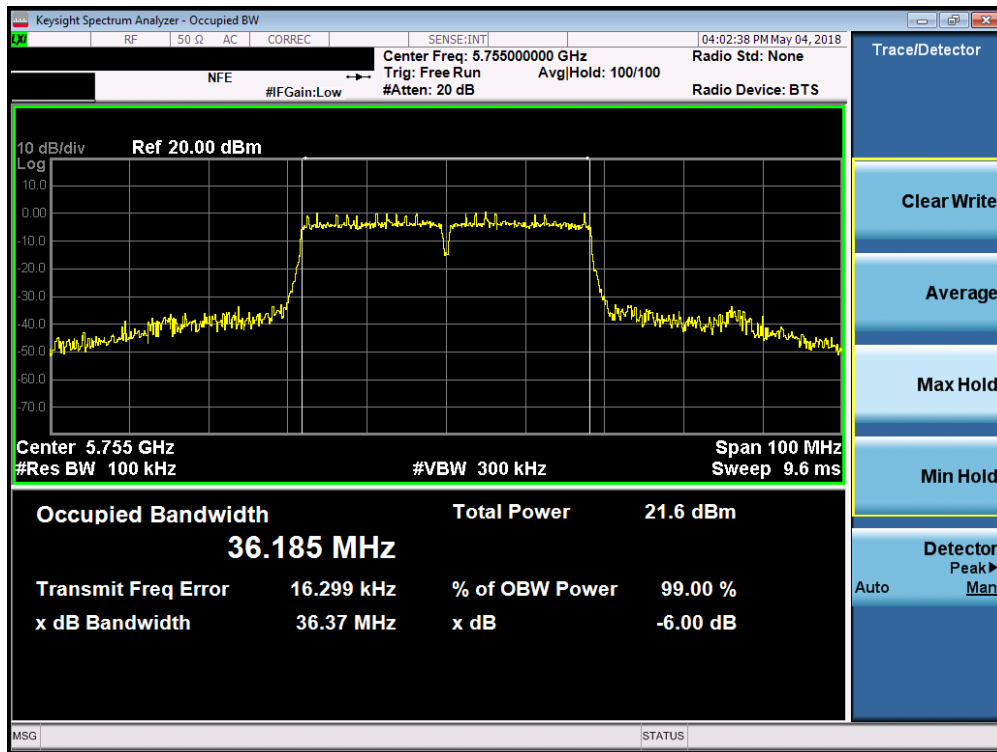
Plot 7-65. 6dB Bandwidth Plot (40MHz BW 802.11n (UNII Band 3) – Ch. 151)
