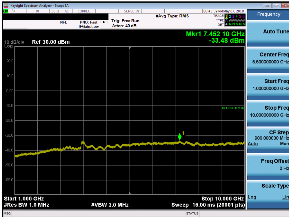
Plot 7-21. Conducted Spurious Plot (LTE B26 – 5.0MHz QPSK – RB Size 1, RB Offset 0 – High Channel)
