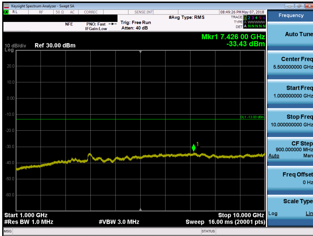
Plot 7-18. Conducted Spurious Plot (LTE B26 – 5.0MHz QPSK – RB Size 1, RB Offset 0 – Low Channel)
