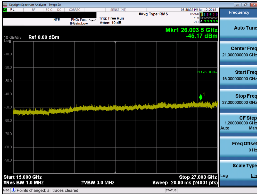
Plot 7-362. Conducted Spurious Plot (Band 41 – 20.0MHz QPSK – PCC 1/99 SCC 1/0 – High Channel)
