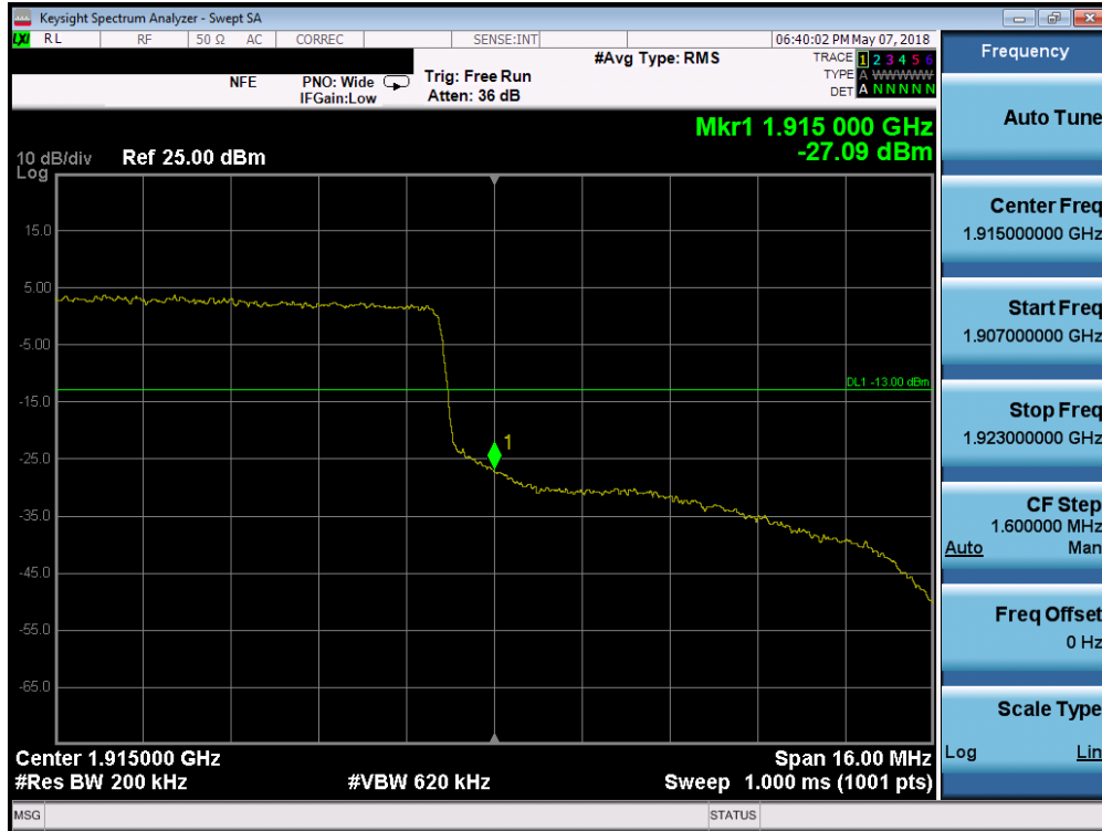
Plot 7-246. Upper Band Edge Plot (Band 25 - 20.0MHz QPSK - Full RB Configuration)
