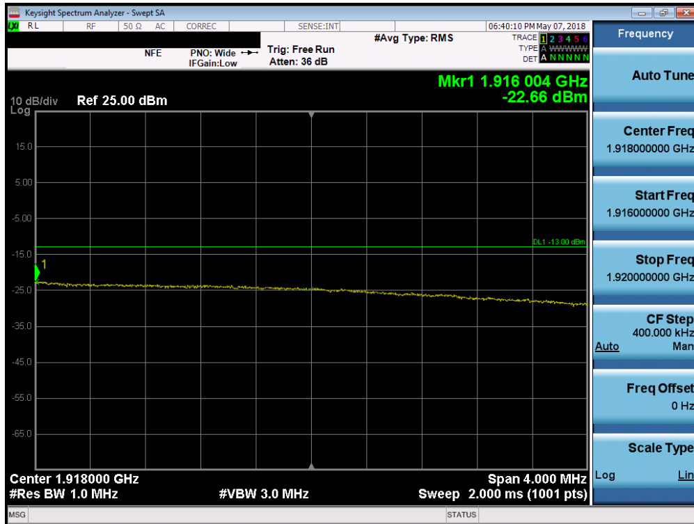
Plot 7-247. Upper Extended Band Edge Plot (Band 25 - 20.0MHz QPSK - Full RB Configuration)
