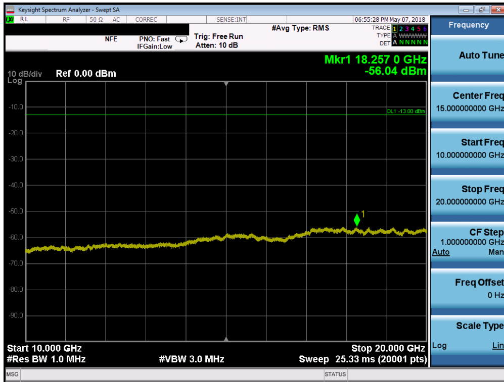
Plot 7-132. Conducted Spurious Plot (Band 25/2 - 5.0MHz QPSK - RB Size 1, RB Offset 0 - Low Channel)
