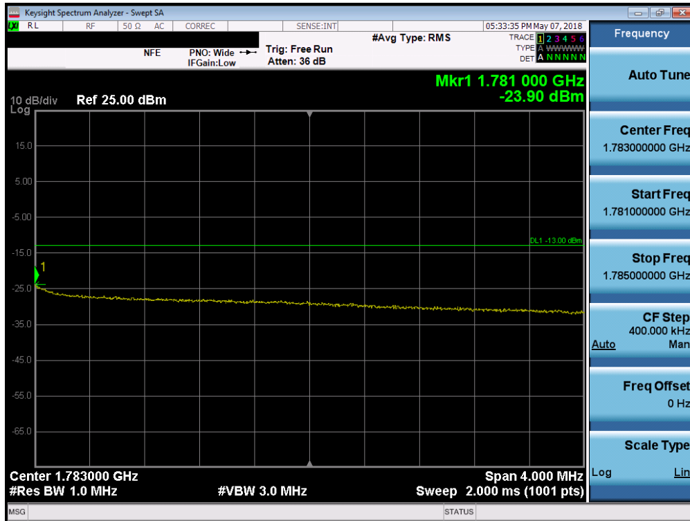
Plot 7-199. Upper Extended Band Edge Plot (Band 66 - 10.0MHz QPSK - Full RB Configuration)
