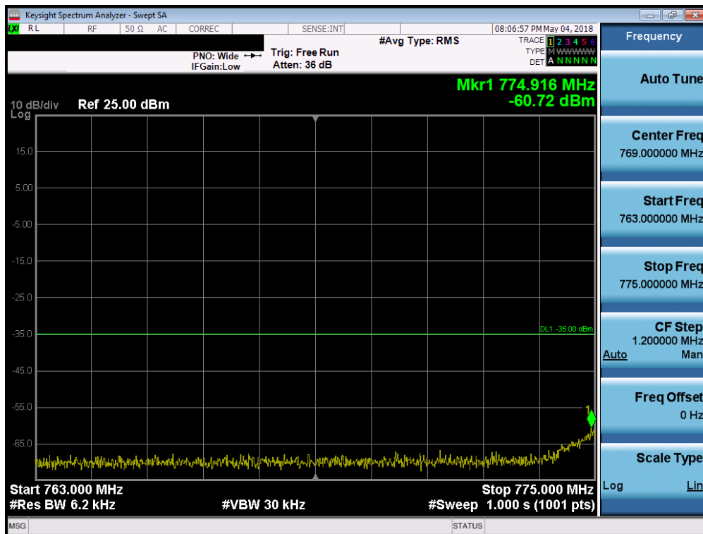
Plot 7-159. Lower Emission Mask Band Edge Plot (Band 13 - 5.0MHz QPSK - Full RB Configuration)
