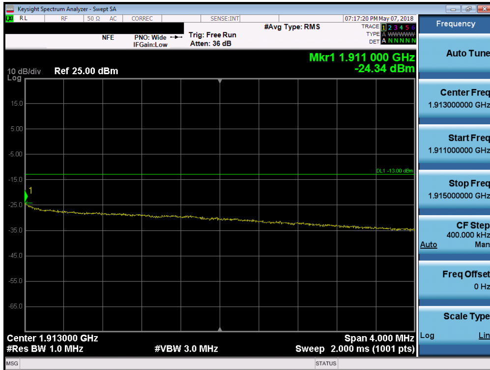
Plot 7-233. Upper Extended Band Edge Plot (Band 2 - 10.0MHz QPSK - Full RB Configuration)
