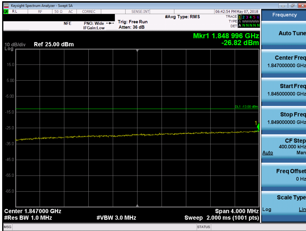
Plot 7-237. Lower Extended Band Edge Plot (Band 25/2 - 15.0MHz QPSK - Full RB Configuration)
