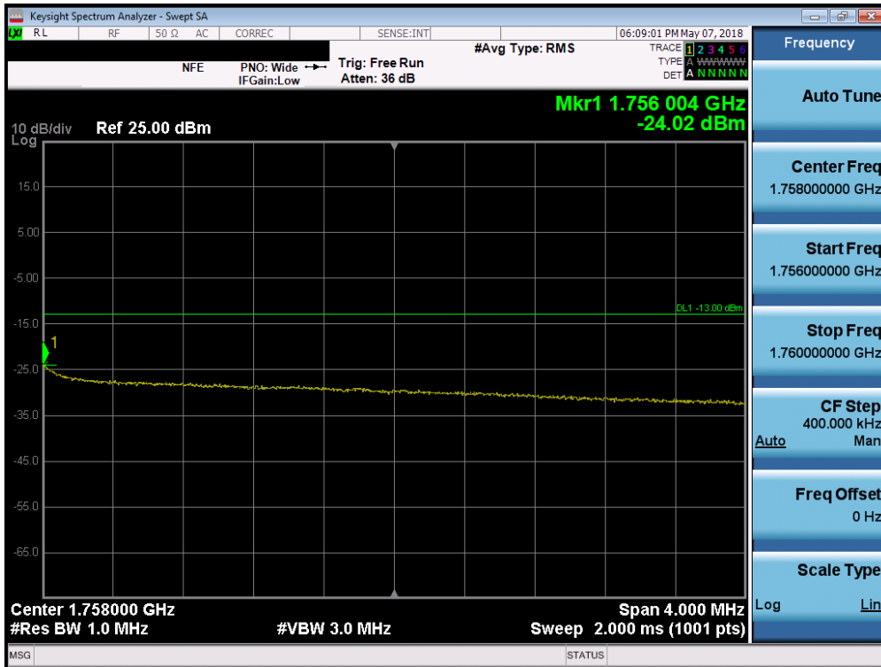
Plot 7-197. Upper Extended Band Edge Plot (Band 4 - 10.0MHz QPSK - Full RB Configuration)
