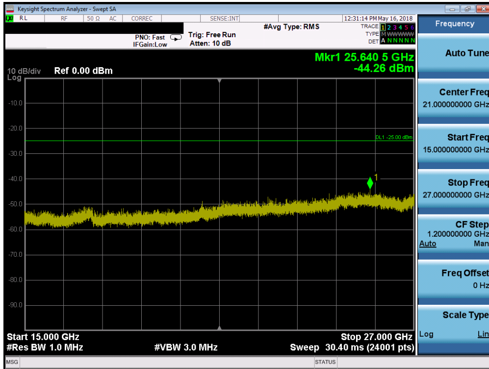
Plot 7-147. Conducted Spurious Plot (Band 41 - 10.0MHz QPSK - RB Size 1, RB Offset 0 - High Channel)
