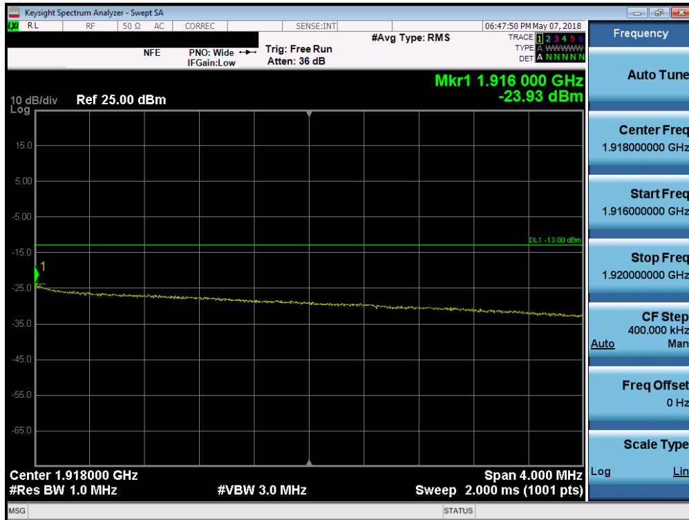
Plot 7-235. Upper Extended Band Edge Plot (Band 25 - 10.0MHz QPSK - Full RB Configuration)
