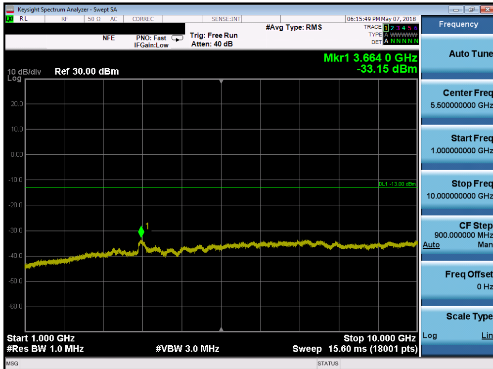
Plot 7-99. Conducted Spurious Plot (Band 12/17 - 5.0MHz QPSK - RB Size 1, RB Offset 0 - Mid Channel)
