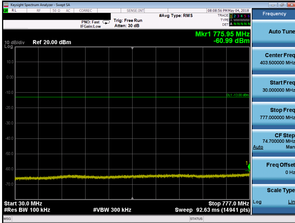
Plot 7-109. Conducted Spurious Plot (Band 13 - 5.0MHz QPSK - RB Size 1, RB Offset 0 - High Channel)
