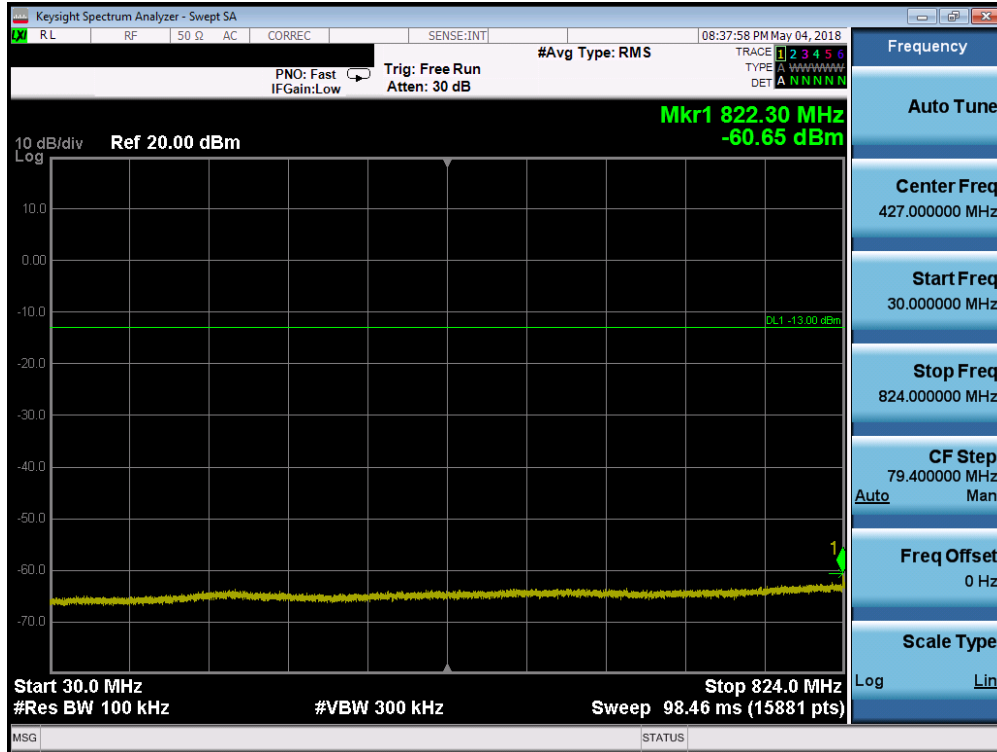
Plot 7-118. Conducted Spurious Plot (Band 26/5 - 5.0MHz QPSK - RB Size 1, RB Offset 0 - High Channel)
