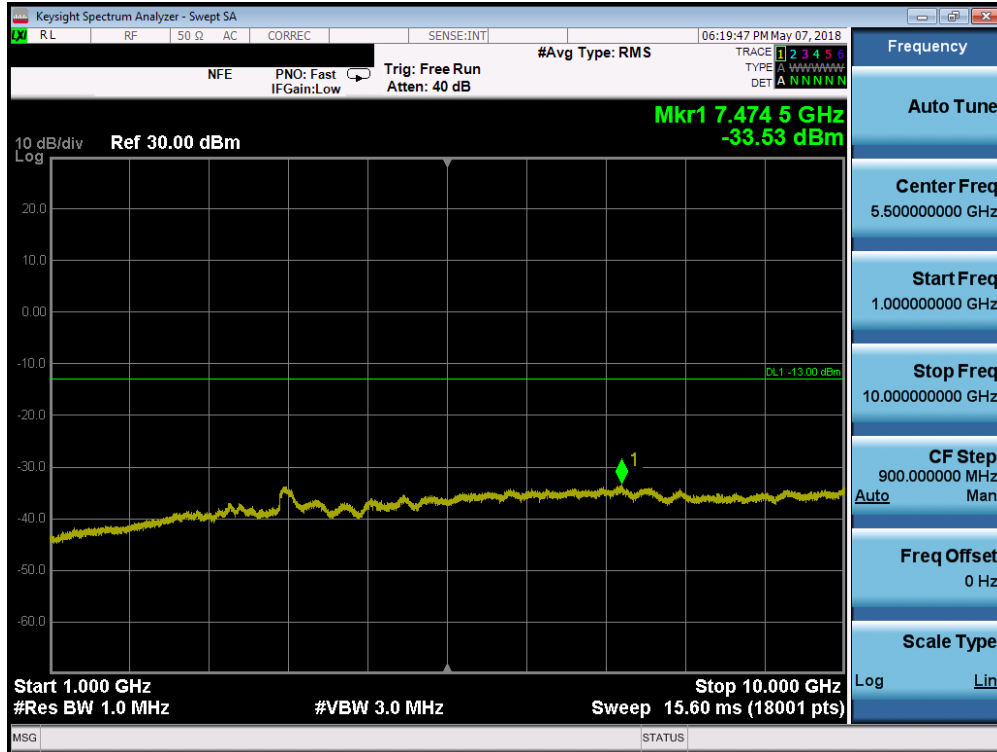
Plot 7-102. Conducted Spurious Plot (Band 12/17 - 5.0MHz QPSK - RB Size 1, RB Offset 0 - High Channel)
