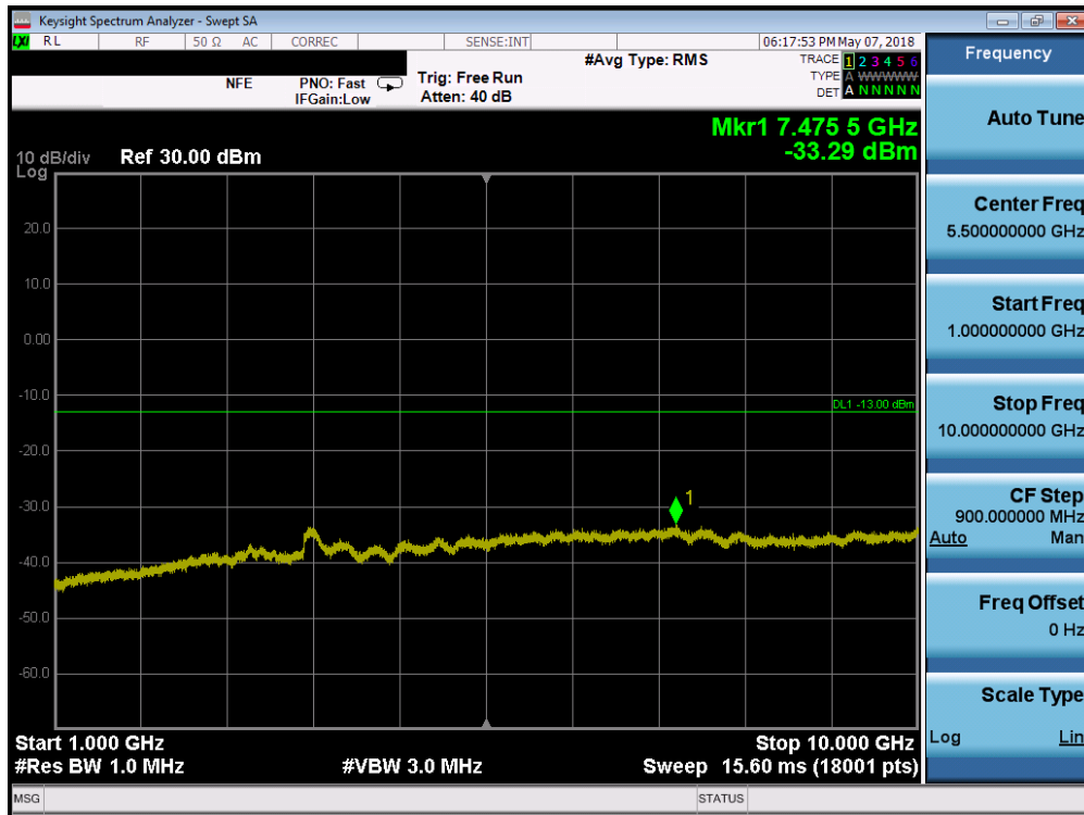
Plot 7-96. Conducted Spurious Plot (Band 12/17 - 5.0MHz QPSK - RB Size 1, RB Offset 0 - Low Channel)
