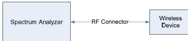
Figure 7-1. Test Instrument & Measurement Setup
