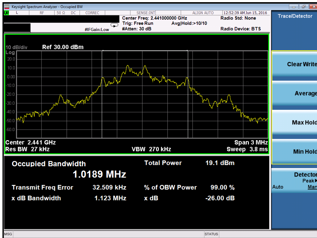
Plot 7-1. Occupied Bandwidth Plot (ANT+ – Ch. 39)
