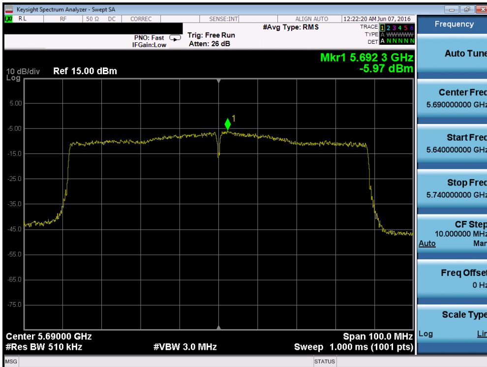
Plot 7-143. Power Spectral Density Plot (80MHz BW 802.11ac (UNII Band 2C) – Ch. 138)
