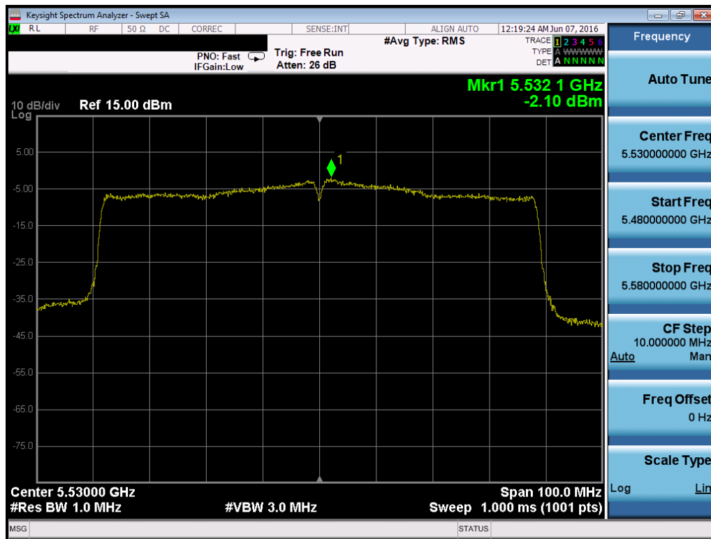
Plot 7-141. Power Spectral Density Plot (80MHz BW 802.11ac (UNII Band 2C) – Ch. 106)
