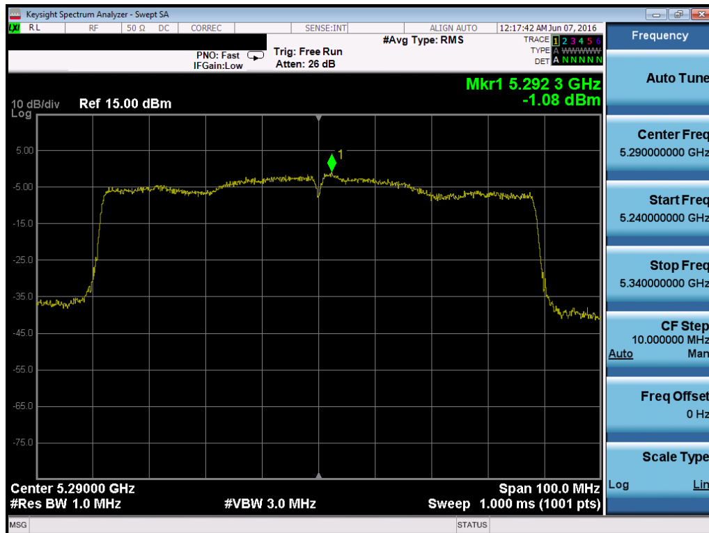
Plot 7-131. Power Spectral Density Plot (80MHz BW 802.11ac (UNII Band 2A) – Ch. 58)
