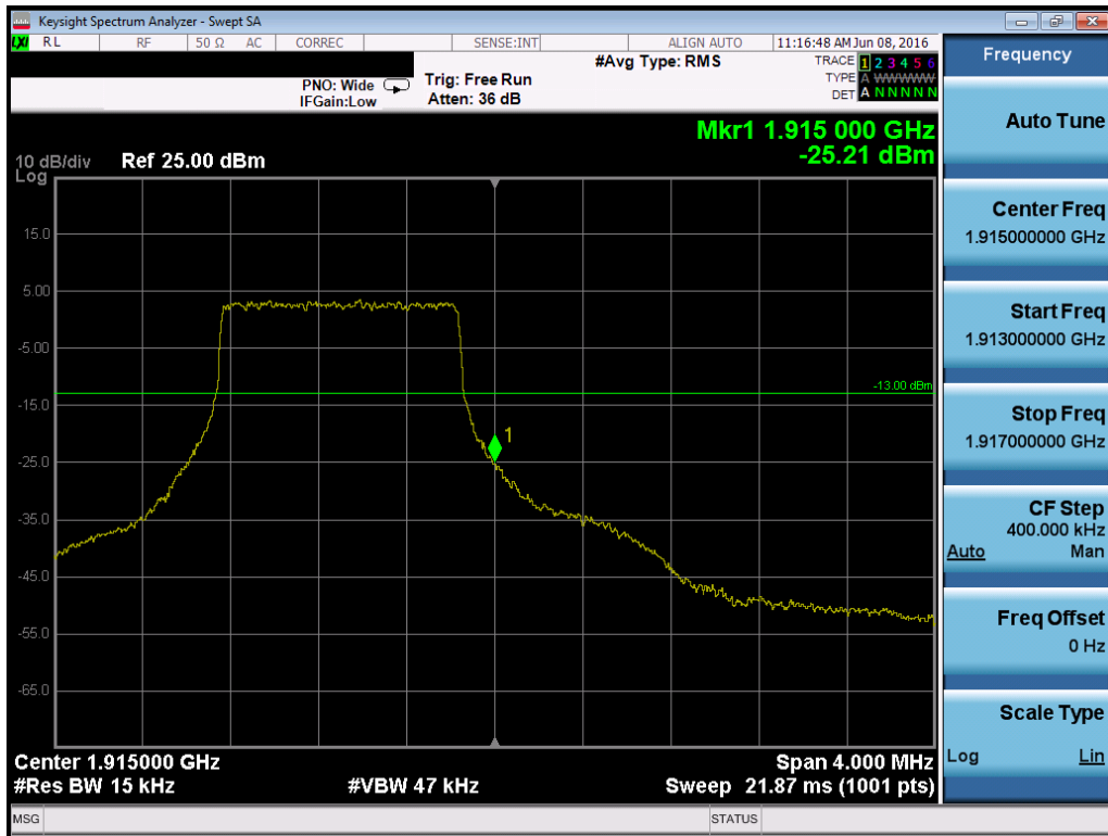
Plot 7-148. Upper Band Edge Plot (Band 25 – 1.4MHz QPSK – RB Size 6)
