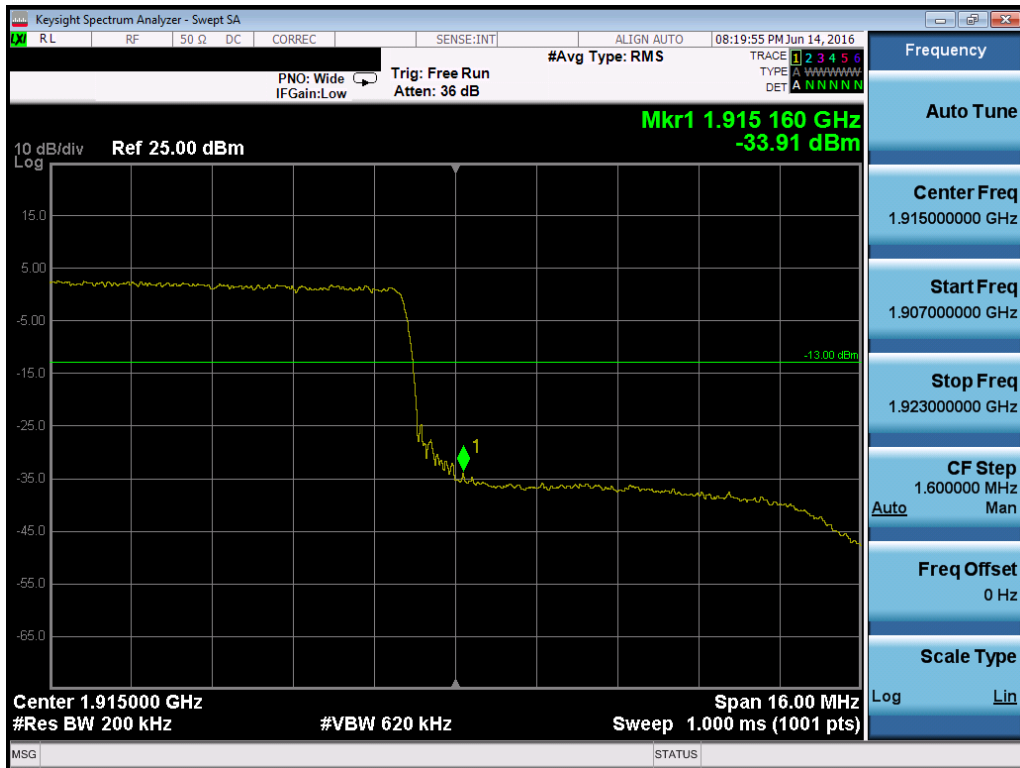
Plot 7-168. Upper Band Edge Plot (Band 25 – 20.0MHz QPSK – RB Size 100)
