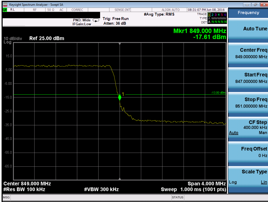
Plot 7-115. Upper Band Edge Plot (Band 5/26 – 3.0MHz QPSK – RB Size 15)
