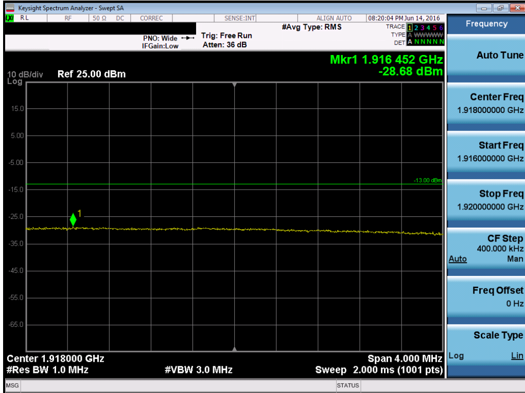
Plot 7-169. Upper Extended Band Edge Plot (Band 25 – 20.0MHz QPSK – RB Size 100)
