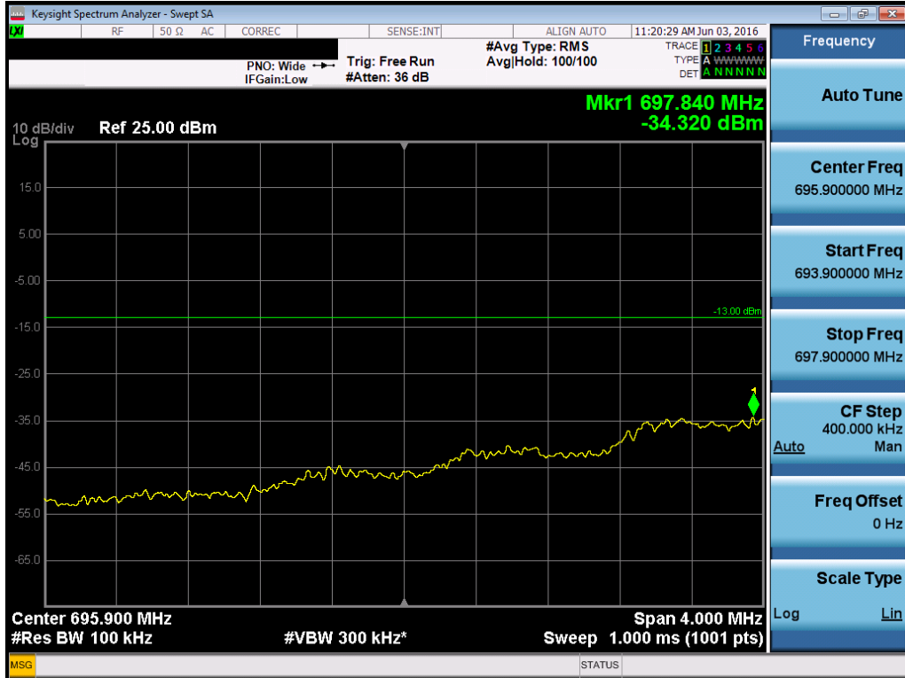
Plot 7-97. Lower Extended Band Edge Plot (Band 12 – 1.4MHz QPSK – RB Size 6)
