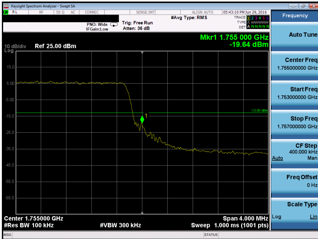
Plot 7-132. Upper Band Edge Plot (Band 4 - 5.0MHz QPSK - RB Size 25)
