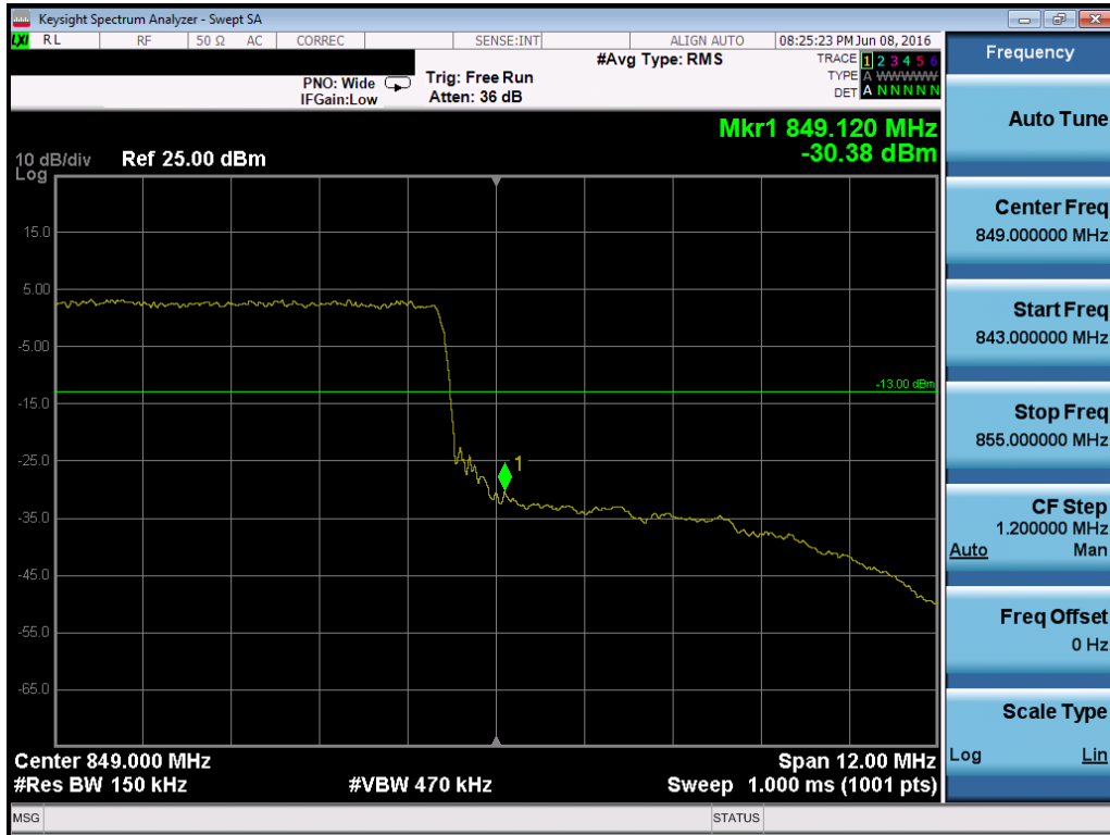
Plot 7-121. Upper Band Edge Plot (Band 26 – 15.0MHz QPSK – RB Size 50)
