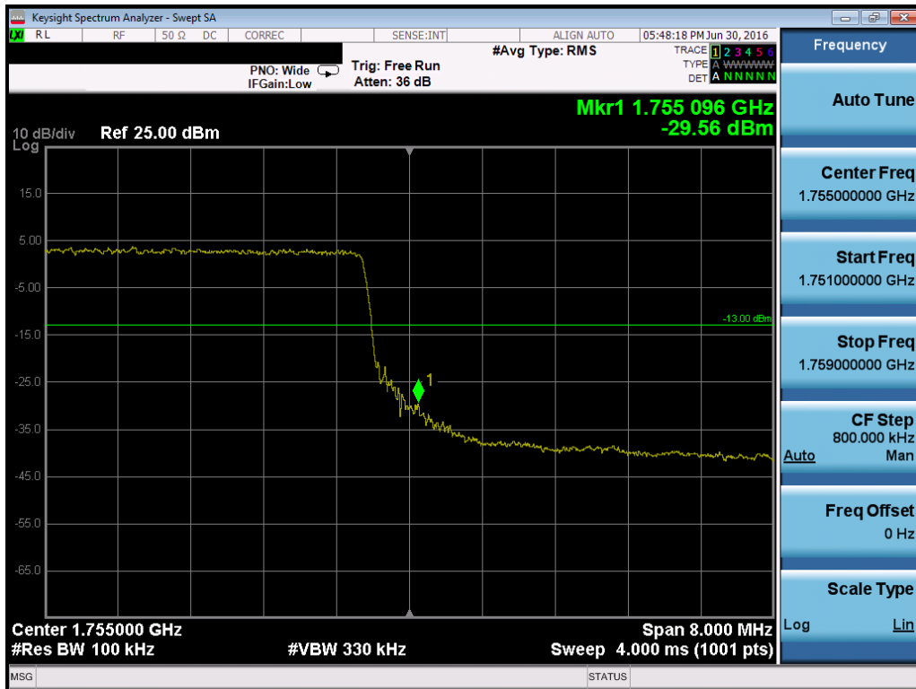
Plot 7-136. Upper Band Edge Plot (Band 4 – 10.0MHz QPSK – RB Size 50)
