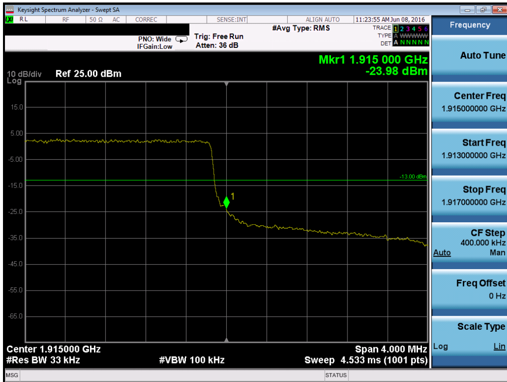
Plot 7-152. Upper Band Edge Plot (Band 25 – 3.0MHz QPSK – RB Size 15)
