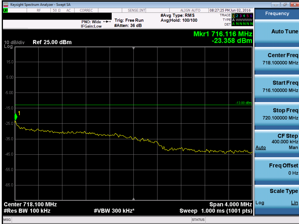
Plot 7-103. Upper Extended Band Edge Plot (Band 12 – 3.0MHz QPSK – RB Size 15)
