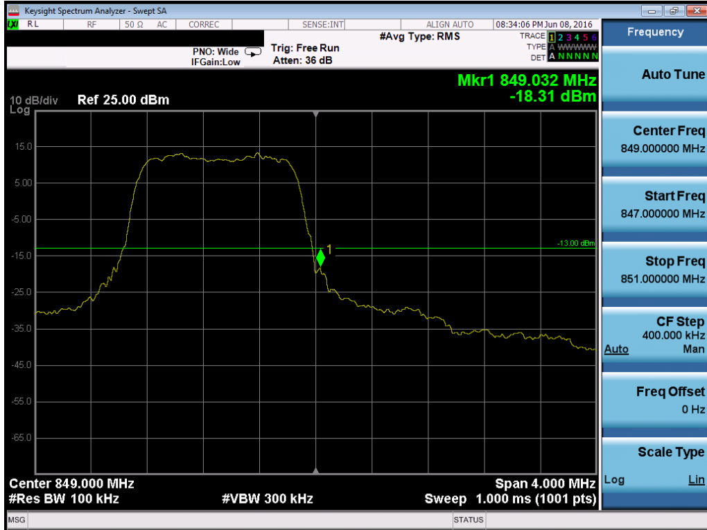
Plot 7-113. Upper Band Edge Plot (Band 5/26 – 1.4MHz QPSK – RB Size 6)
