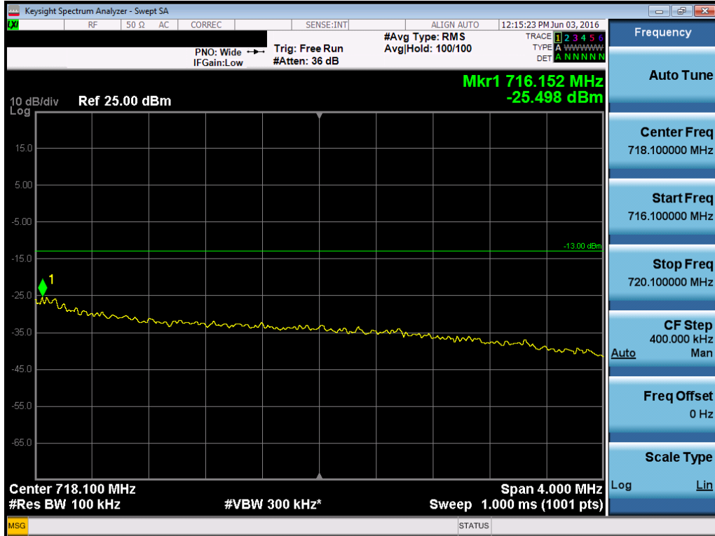
Plot 7-107. Upper Extended Band Edge Plot (Band 12/17 – 5.0MHz QPSK – RB Size 25)
