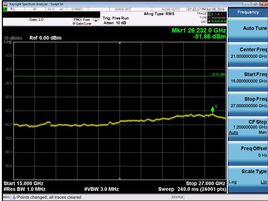
Plot 7-95. Conducted Spurious Plot (Band 41 – 20.0MHz QPSK – RB Size 1, RB Offset 0 – High Channel)
