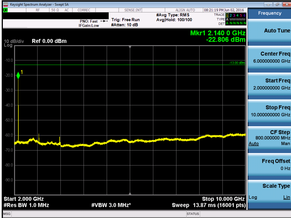
Plot 7-59. Conducted Spurious Plot (Band 12/17 – 5.0MHz QPSK – RB Size 1, RB Offset 0 – High Channel)
