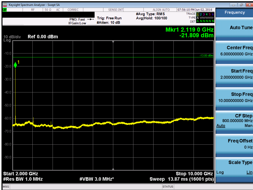
Plot 7-56. Conducted Spurious Plot (Band 12/17 – 5.0MHz QPSK – RB Size 1, RB Offset 0 – Mid Channel)
