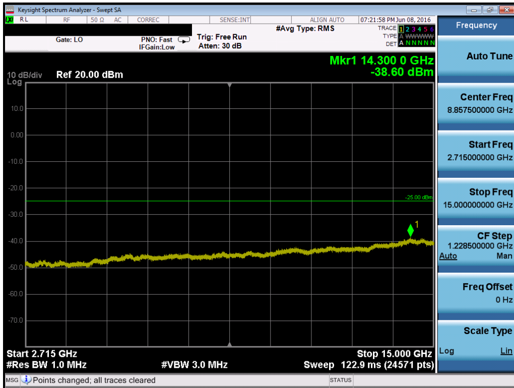
Plot 7-94. Conducted Spurious Plot (Band 41 – 20.0MHz QPSK – RB Size 1, RB Offset 0 – High Channel)
