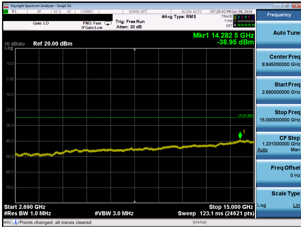
Plot 7-88. Conducted Spurious Plot (Band 41 – 20.0MHz QPSK – RB Size 1, RB Offset 0 – Low Channel)
