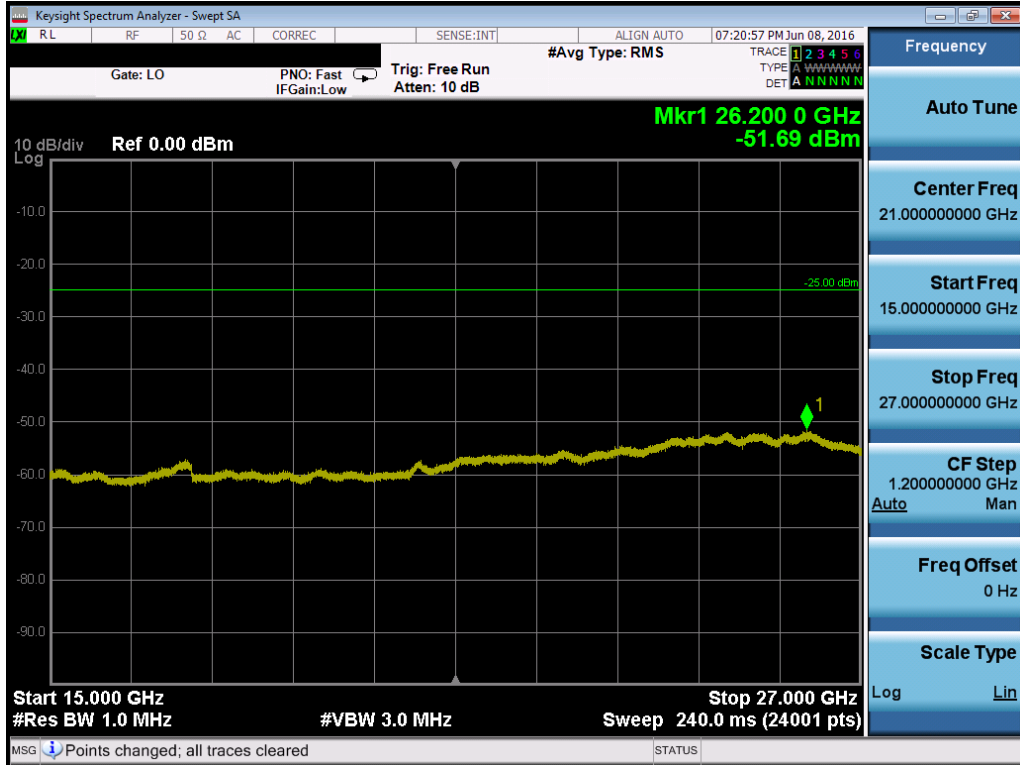
Plot 7-89. Conducted Spurious Plot (Band 41 – 20.0MHz QPSK – RB Size 1, RB Offset 0 – Low Channel)
