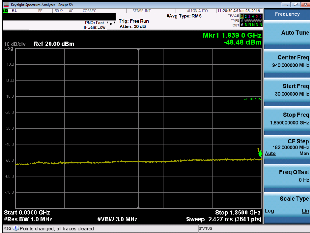
Plot 7-81. Conducted Spurious Plot (Band 2/25 – 5.0MHz QPSK – RB Size 1, RB Offset 0 – Mid Channel)
