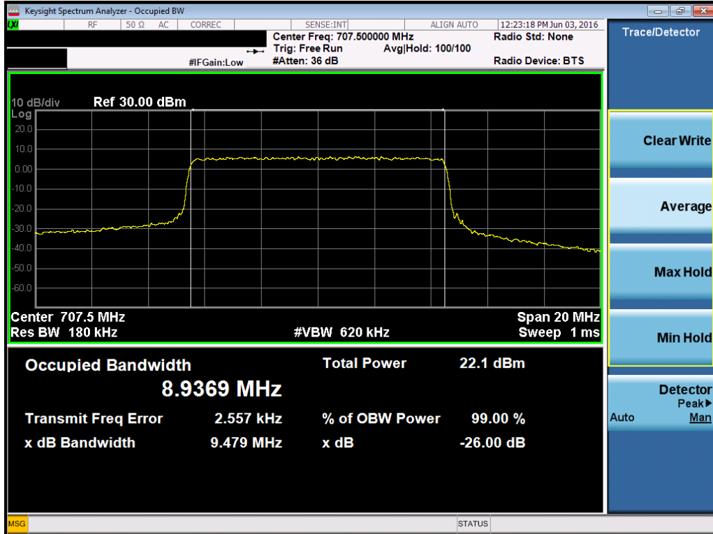
Plot 7-7. Occupied Bandwidth Plot (Band 12/17 – 10.0MHz QPSK – RB Size 50)
