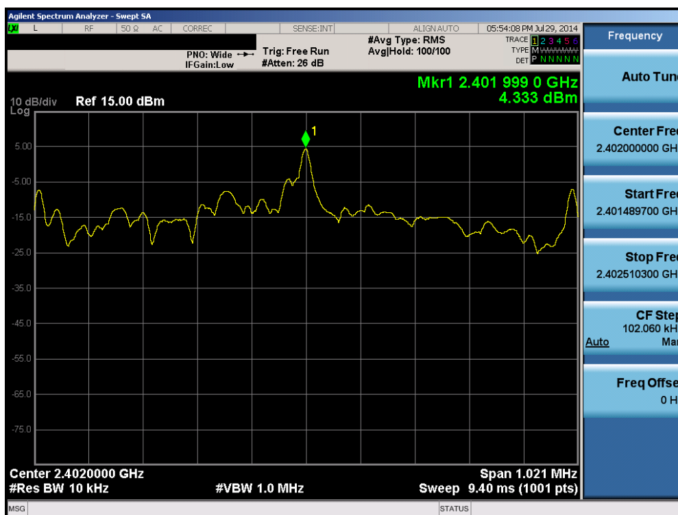
Plot 6-7. Power Spectral Density Plot (Bluetooth (LE) – Ch. 0)
