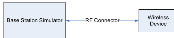
Figure 9-2 Power Measurement Setup
