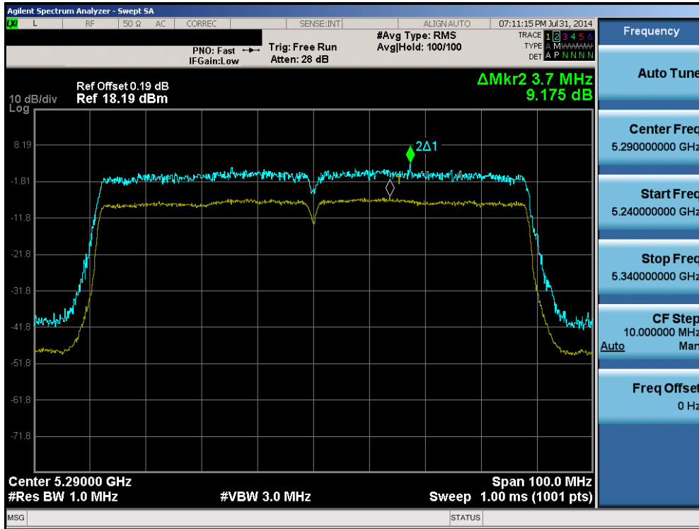
Plot 6-126. Peak Excursion Ratio Plot (80MHz BW 802.11ac (UNII Band 2A) – Ch. 58)
