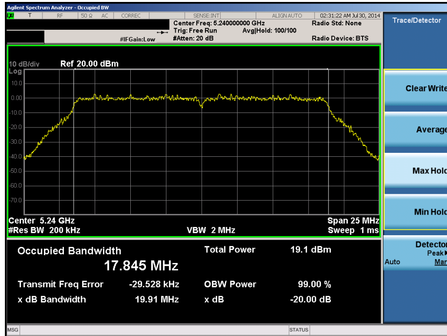
Plot 6-30. 20dB Bandwidth Plot (20MHz BW 802.11n (UNII Band 1) – Ch. 48)
