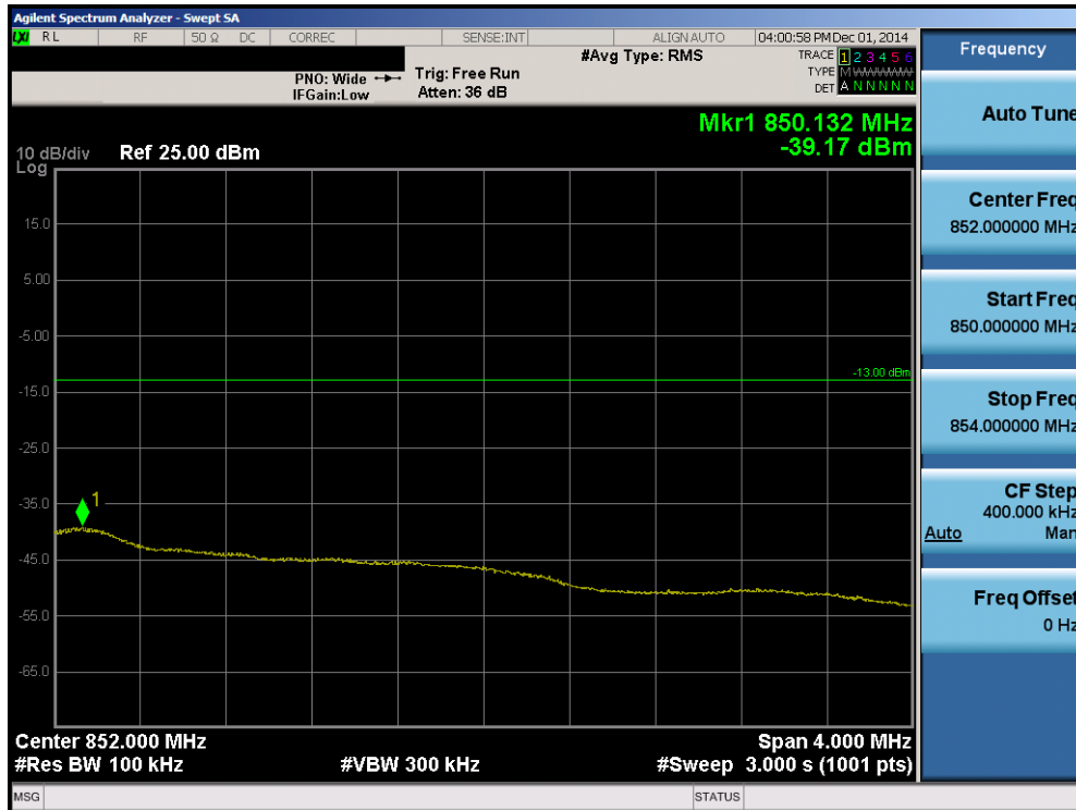
Plot 6-38. Upper Extended Band Edge Plot (Band 5 – Band 5 – 3.0MHz QPSK – RB Size 15)
