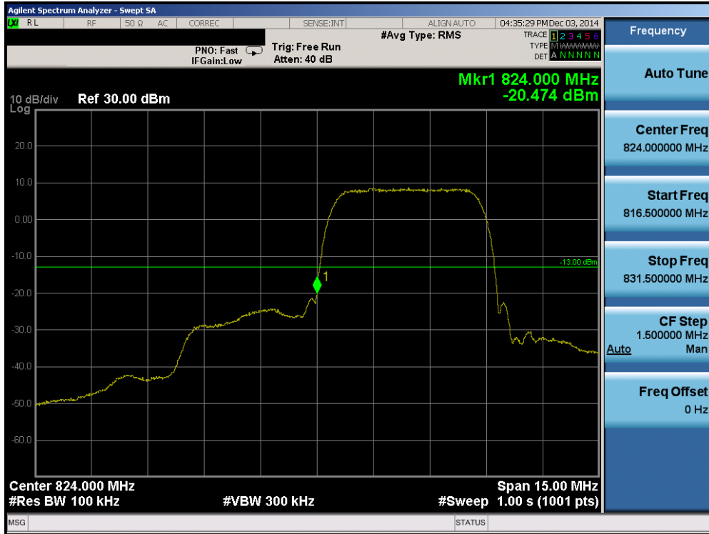
Plot 6-24. Band Edge Plot (Cellular WCDMA Mode – Ch. 4132)
