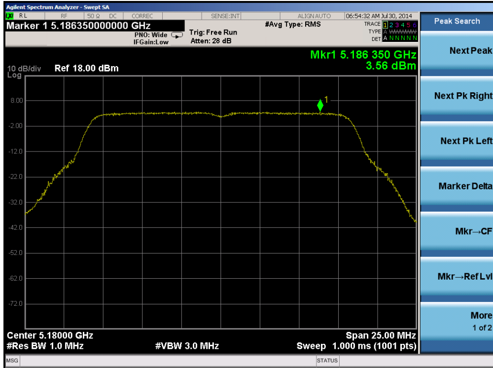
Plot 6-68. Peak Power Spectral Density Plot (802.11a (UNII Band 1) – Ch. 36)
