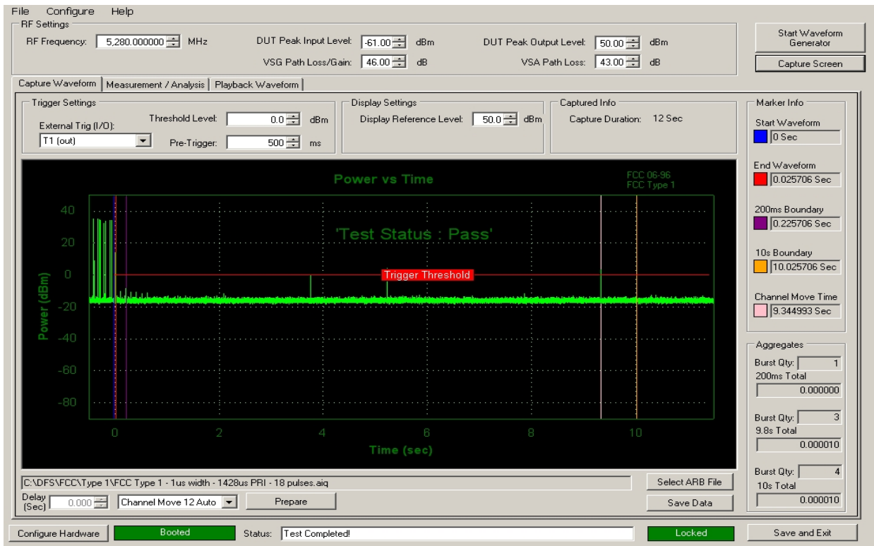
Figure 5-1. Band 2A Move Time and Aggregate Time
