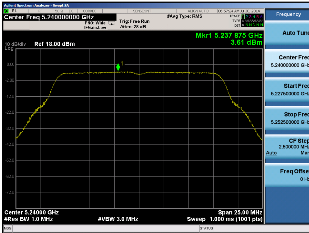
Plot 6-70. Peak Power Spectral Density Plot (802.11a (UNII Band 1) – Ch. 48)
