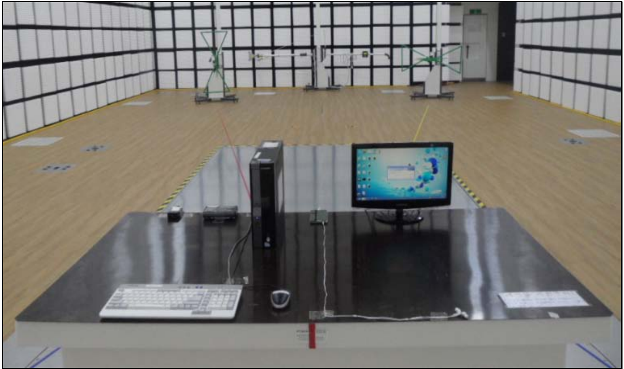
[ Radiated Disturbance for Below 1 GHz – Front ]
