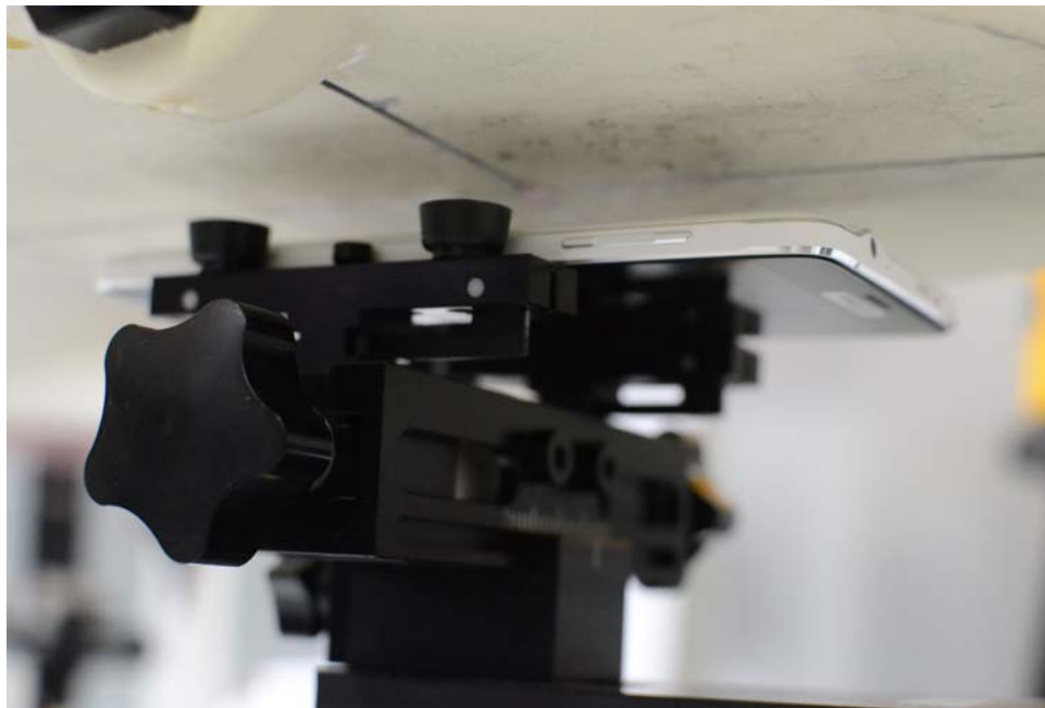
SAR Test Setup Photo 8: Back Side at 1.5 cm with Standard Cover
