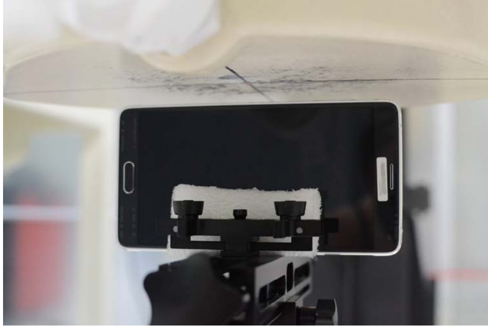
SAR Test Setup Photo 23: Left Edge at 1.0 cm with Standard Cover
