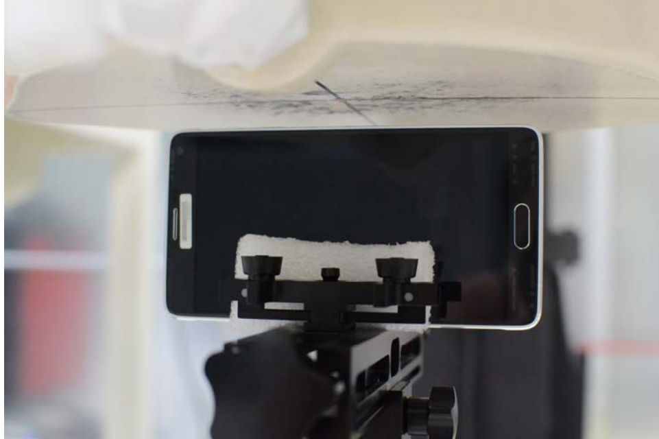
SAR Test Setup Photo 21: Right Edge at 1.0 cm with Standard Cover
