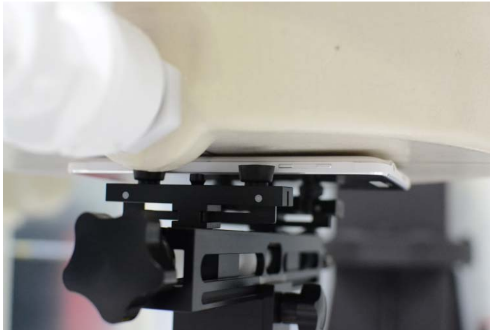
SAR Test Setup Photo 12: Back side at 0.0 cm with Standard Cover
