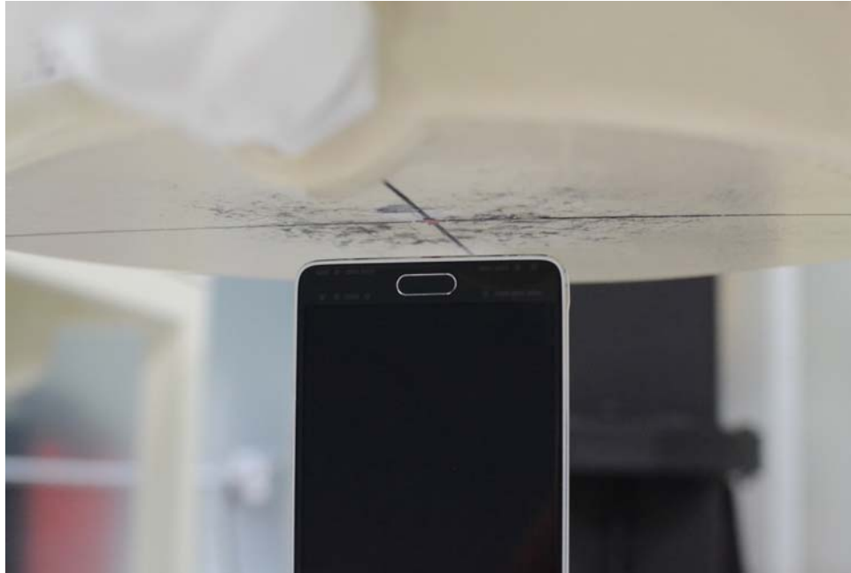
SAR Test Setup Photo 19: Bottom Edge at 1.0 cm with Standard Cover
