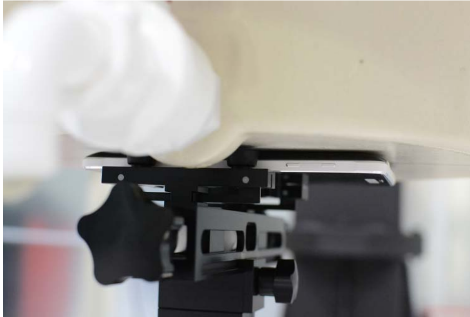
SAR Test Setup Photo 13: Back Side at 0.0 cm with Wireless Charging Cover
