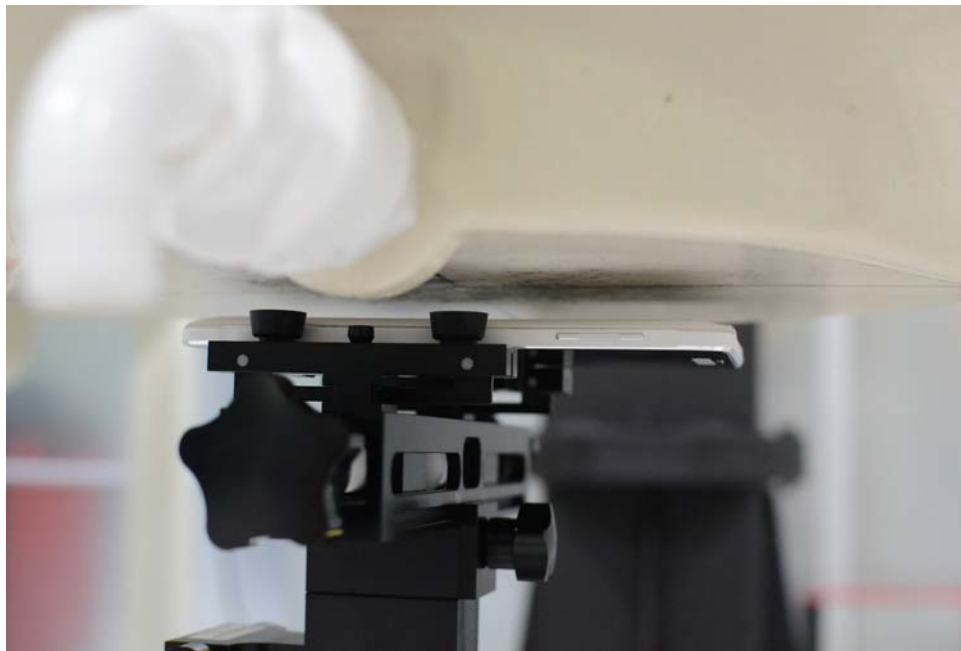
SAR Test Setup Photo 10: Back Side at 1.0 cm with Standard Cover
