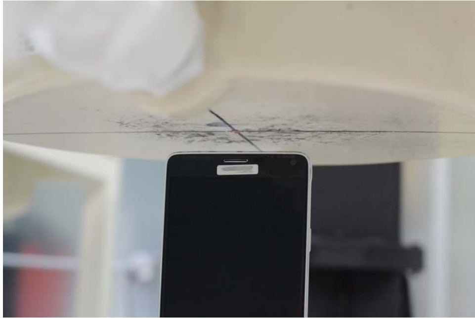
SAR Test Setup Photo 17: Top Edge at 1.0 cm with Standard Cover
