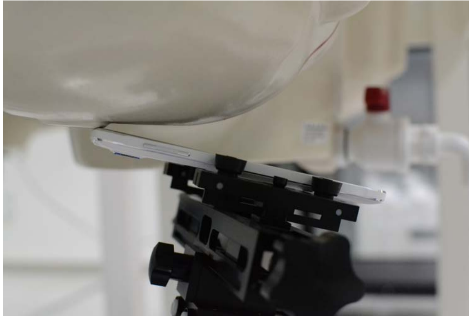
SAR Test Setup Photo 3: Right Tilt with Standard Cover
