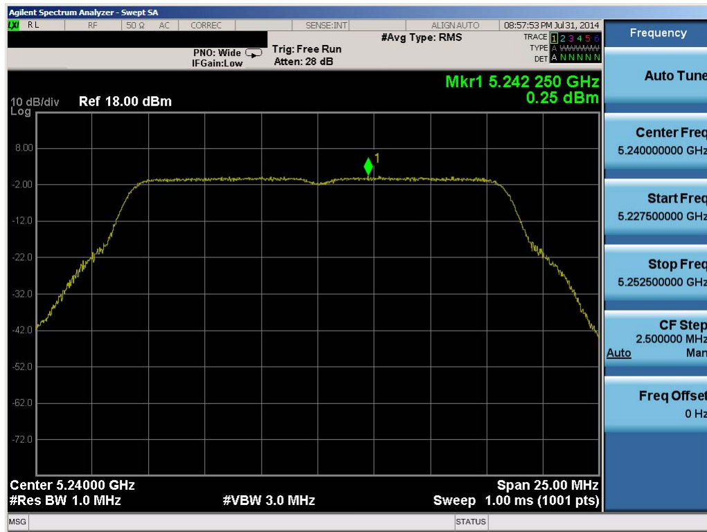
Plot 6-71. Peak Power Spectral Density Plot (802.11a (UNII Band 1) – Ch. 48)
