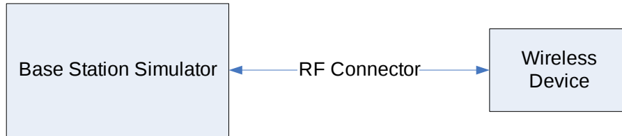
Figure 9-1 Power Measurement Setup
