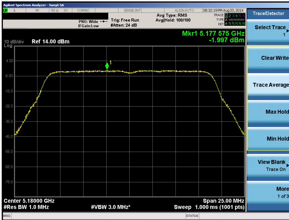
Plot 6-127. Peak Power Spectral Density Plot Antenna 2 - (20MHz BW 802.11n (UNII Band 1) – Ch. 140)
