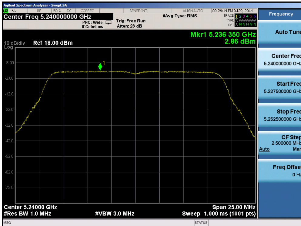
Plot 6-73. Peak Power Spectral Density Plot (20MHz BW 802.11n (UNII Band 1) – Ch. 48)
