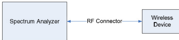
Figure 6-1. Test Instrument & Measurement Setup
