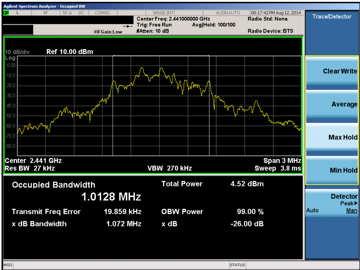
Plot 6-1. Occupied Bandwidth Plot (ANT+ – Ch. 39)
